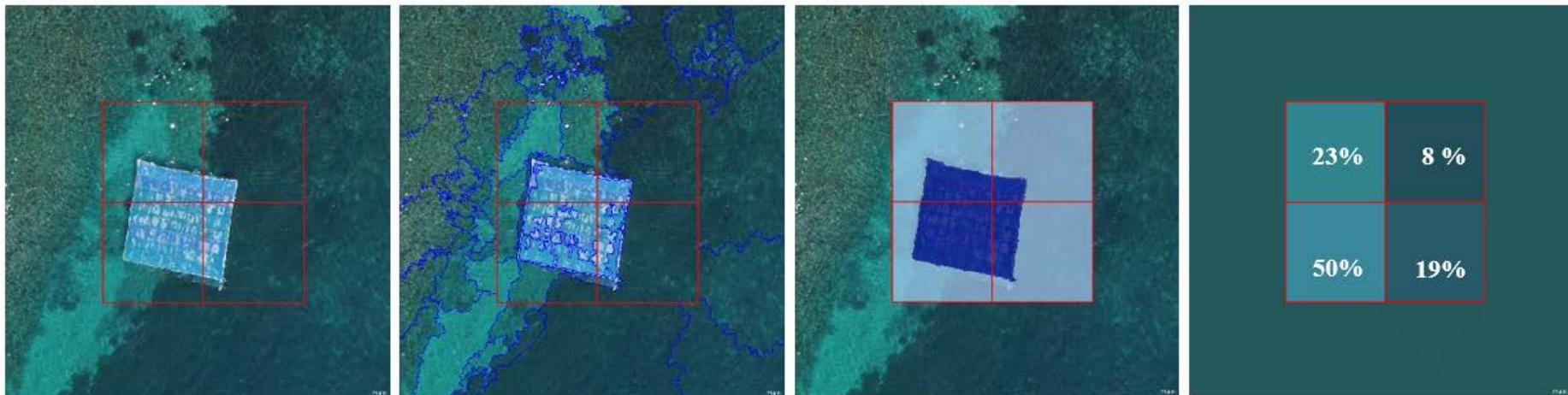
Percentage plastic coverage calculation for each Sentinel-2 pixel using the A5100 orthophotomap
