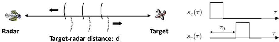
Figure 1.1. Principle of a radar measurement, with s_e(\tau) being the emitted signal and s_r(\tau) being the response of an object
