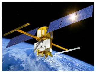
SWOT (Surface Water Ocean Topography) is envisioned for 2020 in a joint project including Nasa and Cnes. It would combine the concepts of WaTER (Water and Terrestrial Elevation Recovery) and the Hydrosphere Mapper missions into a single one to address the objectives of both land hydrology and oceanography. The technology for Swot should be a Ka-band Radar INterferometer (KaRIN, 0.86 cm wavelength).
