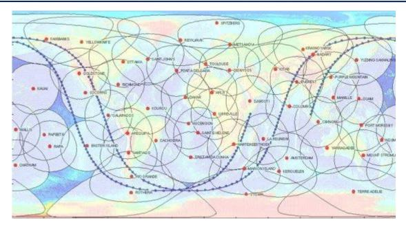
Figure 7.47. The DORIS network of orbitography beacons and their spatial coverage from Jason-1's orbit
