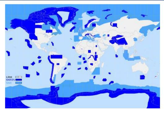
Figure 7.75. Surfaces operated by the 3 modes of Siral (also available on Google Earth, download the kml <u>here</u>). Credits ESA.
