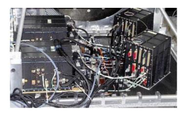
*Figure 7.64.* Poseidon-2 being integrated on Jason-1. Poseidon-3 on Jason-2 is similar. (Credits <u>CNES</u>/Alcatel)
