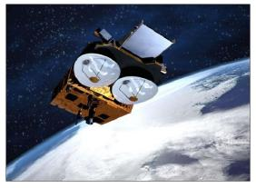
CryoSat-2 is an altimetry satellite built by the European Space Agency and dedicated to polar observation. It embarks on a three-and-a half-year mission to determine variations in the thickness of the Earth's continental ice sheets and marine ice cover, and to test the prediction of thinning Arctic ice due to global warming.
