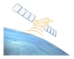
Altimetry is basically a technique for measuring height. Satellite radar altimetry measures the time taken by a radar pulse to travel from the satellite antenna to the surface and back to the satellite receiver. Moreover, this measurement yields a wealth of other information that can be used for a wide range of applications.
