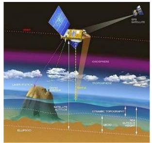
Figure 5.3. The principle of altimetry (Credits CNES/D. Ducros)
