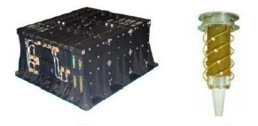
Figure 7.83. SARAL/AltiKa DORIS Receiver Antenna and Instrument
