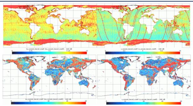
Figure 5.26. Sigma0 in Ku and S band (from Envisat GDR cycle 40) measurements (top over ocean, bottom over lands). Water, ices and lands give very different values of these backscatter coefficients, since those surfaces have different reflexivity. These maps are drawn using the BRAT.
