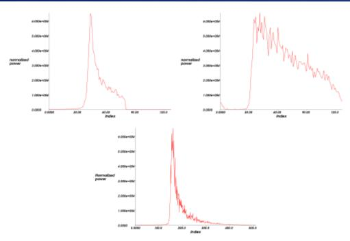
Figure 6.89. Three waveforms over ocean: in SAR mode (left) and, for comparison since it is the most usual shape of a waveform, in LRM mode (middle). (right) A waveform in SAR-In mode over ocean (South of Iceland). The number of gates in the SAR-In mode is 512 (vs 128 in the other two modes).
