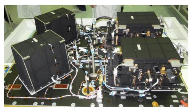
Figure 7.88. Poseidon-3B being integrated on Jason-3 (Credits CNES)
