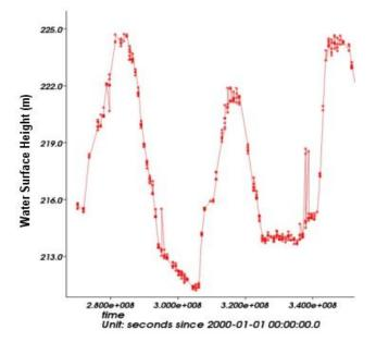
Figure 6.125. Water surface altitude of the Sathanur reservoir from the Pistach "hydro" products, after selection of the data.
