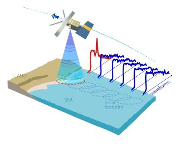
Figure 5.2. Altimeter received waveforms in sea to land transition illustration (COASTALT portal)
