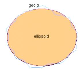
Figure 5.37. Schematic of the Reference ellipsoid with respect to the geoid.
