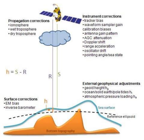
Figure 5.29. Altimetry corrections illustration
