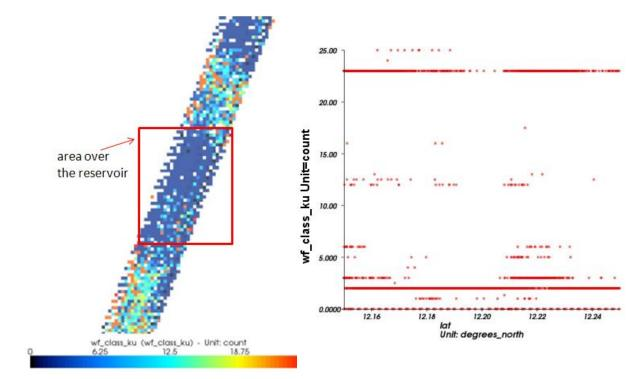
Figure 6.123. Distribution of the waveform classes between latitudes 12.15°N and 12.25°N, along the track (left: as a function of longitude/latitude) and on a diagram (right: as a function of the latitude). The value of each waveform class is detailed in the PISTACH products handbook). Here we mainly see waveform class 2 (peaky) and 23 (multi-peak).
