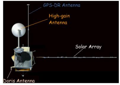
The Topex/Poseidon satellite adaptation was an by Fairchild Space of the existing **Multimission** Modular Spacecraft (MMS) which successfully carried the payloads of the Solar Maximum Mission, Landsat 4 and Landsat 5. The MMS design was modified to meet Topex/Poseidon's
