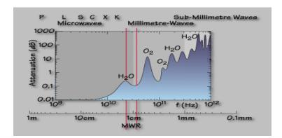
Figure 7.34.Electromagnetic spectrum and MWR frequencies
