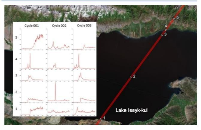
Figure 6.112. Individual waveforms along five given points over the lake Issyk-kul for the three first cycles of OSTM/Jason-2 (maps from Google Earth). X-axis represents the 104 waveforms samples (gates) in Ku-band, so the time. The Y-axis represents the return echo power.
