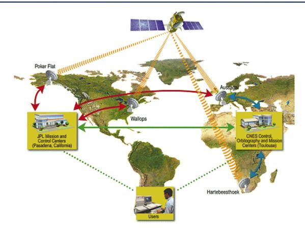
Figure 7.60. Ground Segment components
