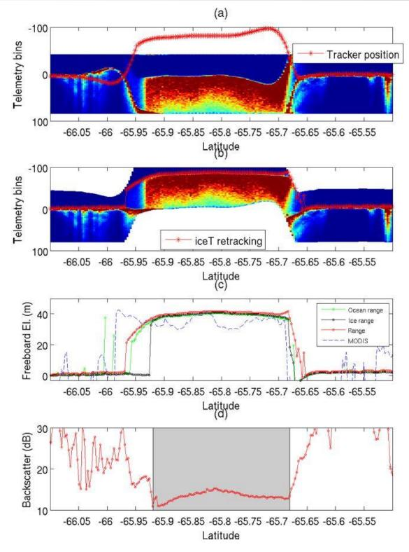
Figure 6.31. Altimeter waveforms for the Envisat pass. The red line indicates the tracker position (a).
