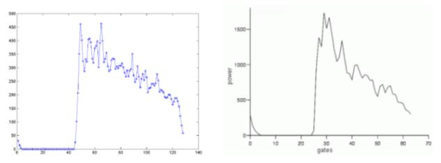
Figure 5.10. Example of real Envisat (left) and Topex (right) waveforms over the ocean.
