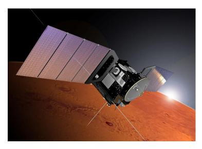
The MARSIS (Mars Advanced Radar for Subsurface and Ionosphere orbital radar Sounding) sounder. onboard ESA's Mars Express spacecraft launched in 2003, was designed to investigate the Martian ionosphere and the geological and hydrological structure of the subsurface, with a particular emphasis on the detection of deep bodies of solid or liquid water
