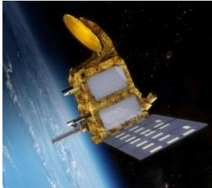
An Isro (Indian Space Research Organization) satellite, Saral (Satellite with ARgos and ALtika), embarks the AltiKa altimeter (working in Ka-band, 35 GHz), built by Cnes, as well as a Doris instrument. Signal frequencies in the Ka-band enables better observation of ice, rain, coastal zones, land masses (forests, etc.), and wave heights.
