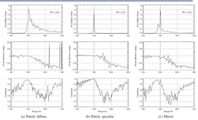
Figure 6.33. CryoSat-2 power waveforms (top row) along with the corresponding phase (middle row) and coherence (bottom row) exhibiting a) purely diffuse behaviour (ice), b) purely specular behaviour (lead) and c) mixed behaviour. The vertical dashed line is the retracking point for the waveform and the pulse peakiness (PP) of each waveform is printed in the top right (Credits T. Armitage)
