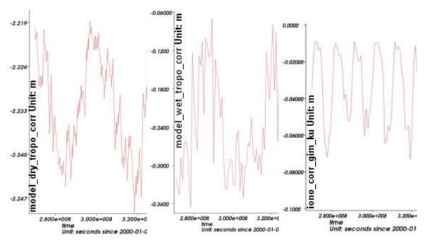
Figure 6.119. Amplitudes in metres of the dry tropospheric correction derived from model (left), of the wet troposheric correction derived from model (middle) and of the ionospheric correction derived from the GIM model (right).
