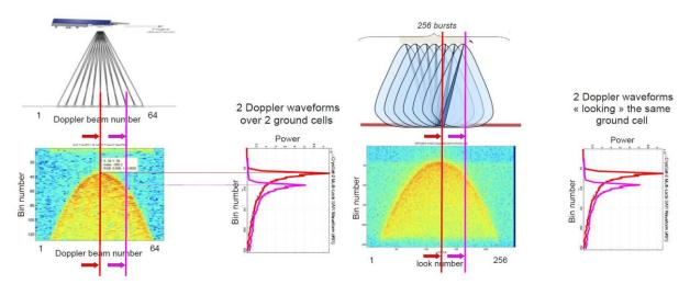
Figure 5.61. Doppler beams obtained from a burst of pulses. Credit: S.Dinardo ESA
