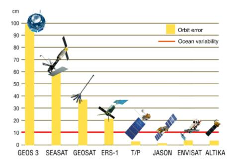
*Figure 7.1. Improvements in measurement accuracy since the first satellite altimetry missions has enabled us to observe ocean variations at close quarters since 1992. (Credits <u>CNES</u>)*
