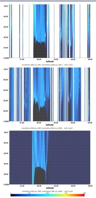
Figure 6.113. Set of juxtaposed waveforms as a function of latitude  $(41^{\circ}N - 45^{\circ}N, pass \#131)$ and as seen from above for the first three cycles of OSTM/Jason-2. Each cycle corresponds to a different tracker: SGT for cycle 001, Median tracker for cycle 002 and Diode+MNT for cycle 003
