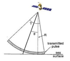
Figure 5.5. Altimeter transmission geometry, R represents the distance from the satellite to the sea surface,  $\gamma$  represents the pointing angle and  $\theta$  the pitch angle
