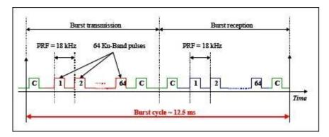
*Figure 5.53. Sentinel-3 transmission pattern. Note that bursts include 2 C-band pulses here. These are used for ionospheric corrections. Credit: ESA*
