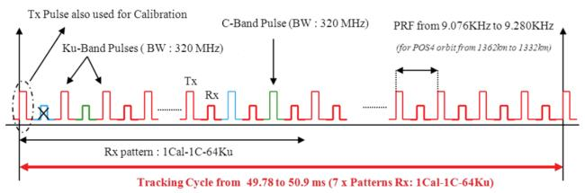
Figure 5.54. Sentinel-6 transmission pattern. Observe that no bursts are present and calibration pulses are also in the same transmission pattern as the Ku- and C-band pulses. Credit: ESA
