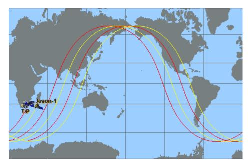
*Figure 7.22.* T/P on its new orbit, situated at one half the Jason-1 track spacing to the west of Jason-1. Cycle 369, which began on Friday 20 September, was the first full cycle in the new orbit. (Credits <u>Aviso</u>)
