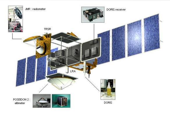
Figure 7.43. Jason 1 instruments
