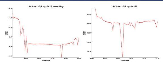
Figure 6.107. Lake level height for the Aral sea without data editing, T/P cycle 010 (left); The measurements over the sea is the "flat" area in the middle of the curve (between, roughly, 59.1° and 60.3°N). Right, a more problematic cycle, cycle 353, for which no clear signal can be seen.
