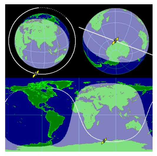
Figure 7.20. Topex/Poseidon orbit
