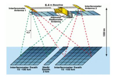
Figure 5.46. How the WSOA altimeter/interferometer works.
