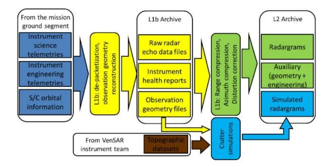
Figure 7.108. Scheme illustrating data processing flow and related data products. Credits EnVision Team.
