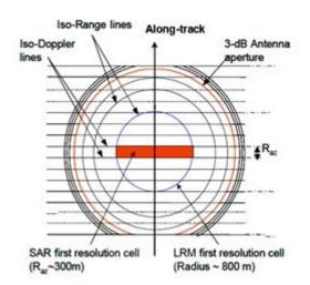
Figure 5.60. SAR Resolution Cell (Credit: TAS-F)
