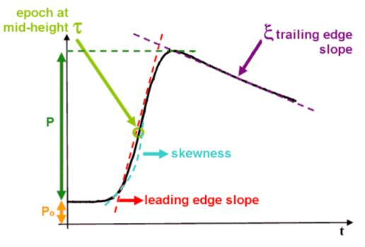
Figure 5.9. Parts of a waveform
