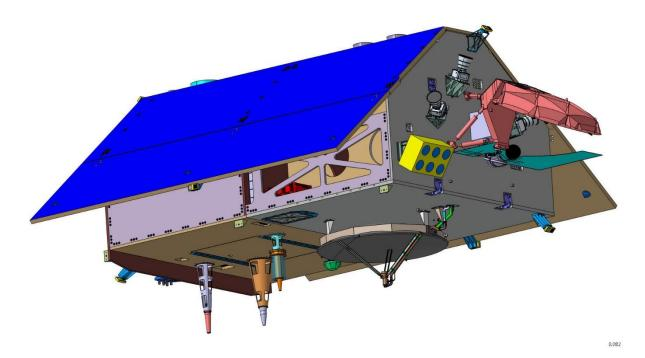
Figure 7.93 Sentinel-6 Satellite and Payloads (Credit: Airbus Defence and Space)
