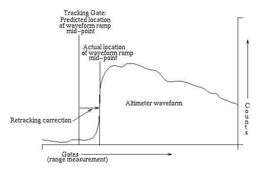
Figure 5.44. Typical ice sheet altimeter waveform illustrating the retracking correction that must be applied to compensate for deviation of the waveform's leading edge from the on-board altimeter tracking gate. (Credits NASA/GSFC)
