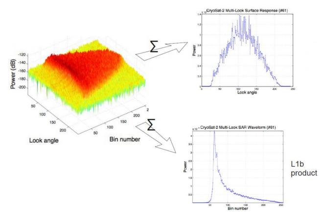
Figure 5.62. Multiple contributions from different bursts conforming to one stack. Credit: S.Dinardo ESA
