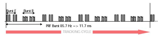
Figure 5.52 CryoSat-2 transmission pattern. Each burst is formed of 64 Ku-band pulses. Credit: ESA.
