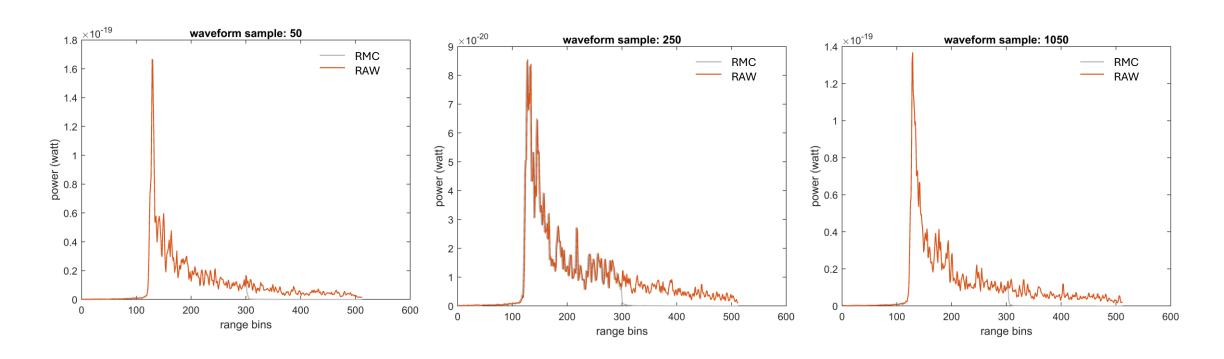
Qualitative analysis demonstrates that signals from both modes align perfectly. The middle panel highlights a minimal shift in the RAW waveform, less than 1/3 of one range bin, which is negligible and is not expected to affect data quality.
