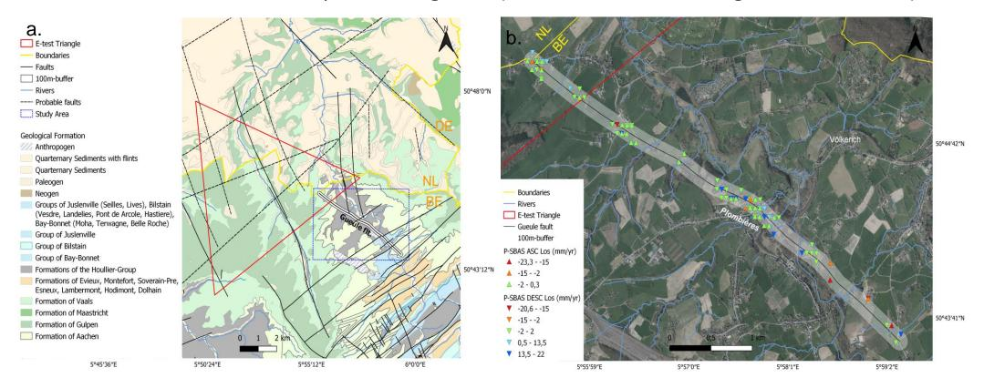
S1 images processed with in ascending track between 2020/12/26 and 2021/07/24 and descending between 2020/12/23 and 2021/07/03 using PSBAS (b)
