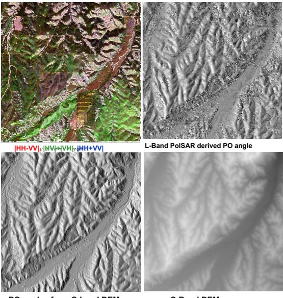
**PO angles derived from DEM of C-Band interferometry**
