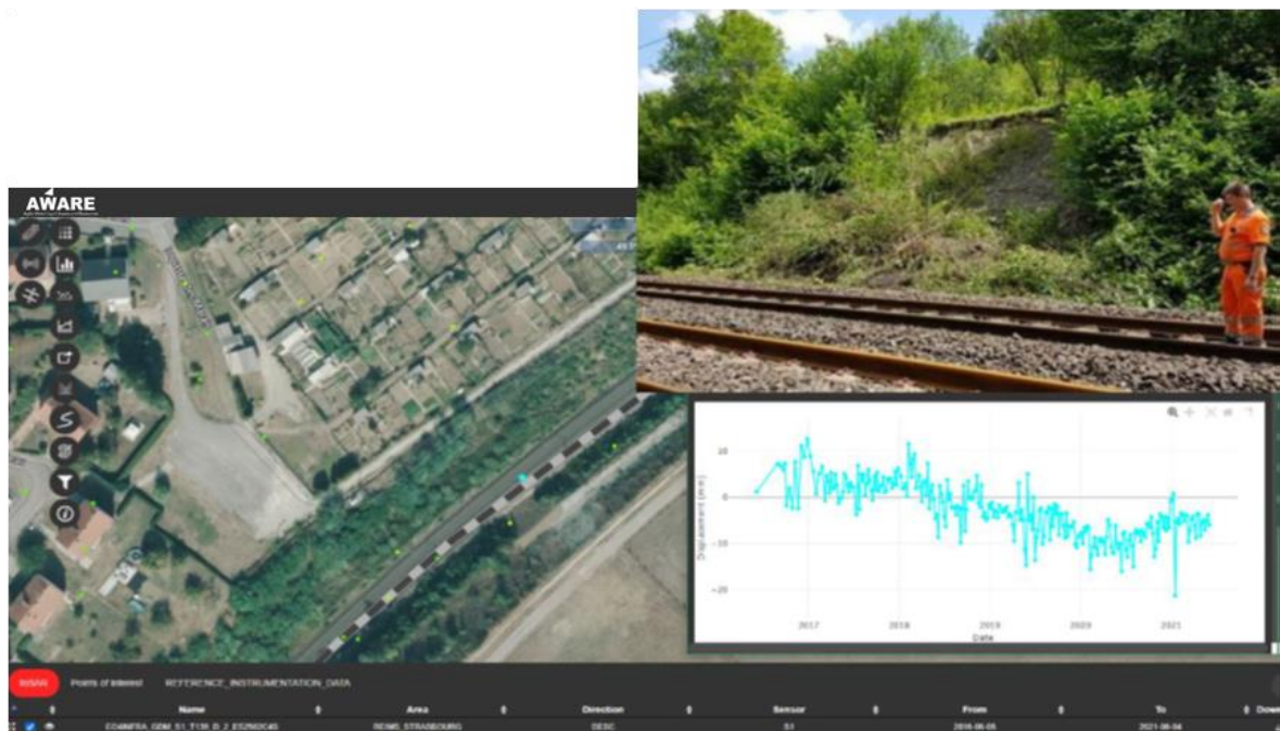
Figure 6: Example of Earthworks monitoring using Medium Resolution Ground Motion map
