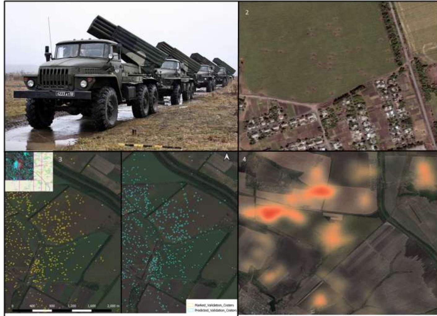
1: BM-21 rocket artillery system 2: Result of rocket artillery shelling 3: Side by side comparison of manually marked craters and UNet detected craters (blue) 4: A kernel density map showing intensity of artillery and rocket shelling across a landscape
