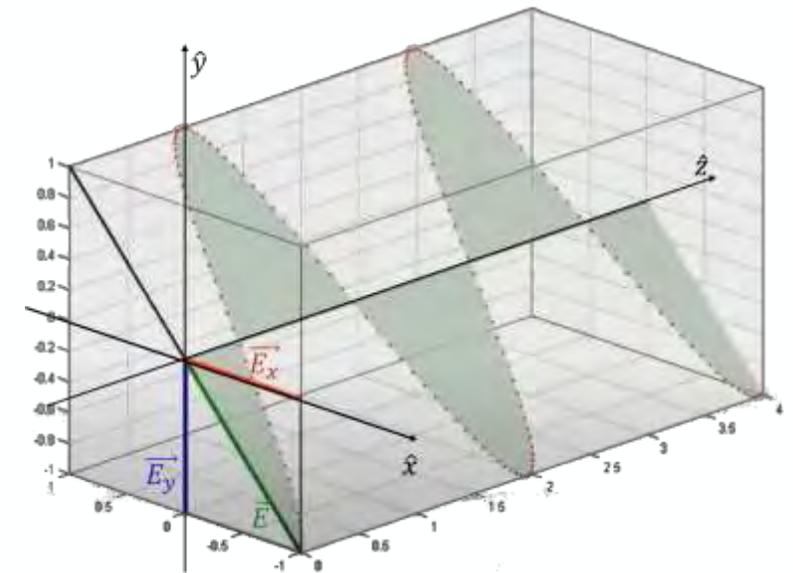
$x, y$  component equal in amplitude and phase
