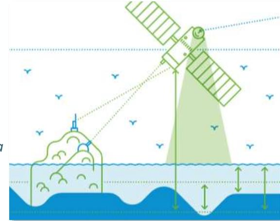
Measures turnaround time delay of short electromagnetic pulse.
