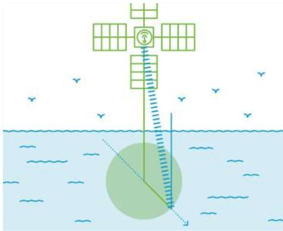
Measures the scattering energy produced while scanning the surface of the Earth.
