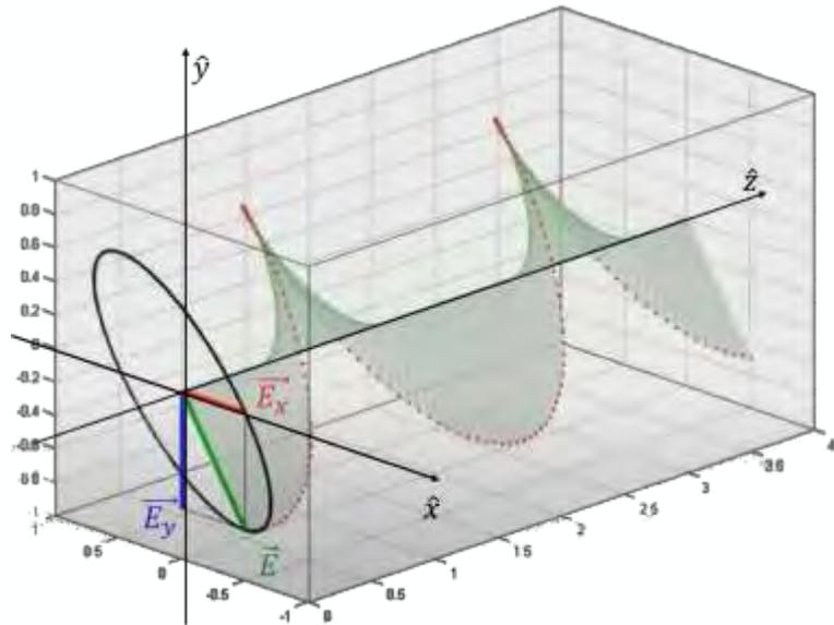
$x, y$  component unequal in amplitude with relative phase  $\neq 0^\circ, 90^\circ$
