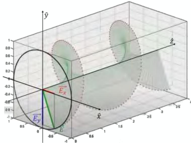
$x, y$  component equal in amplitude with relative phase  $= \pm 90^\circ$
