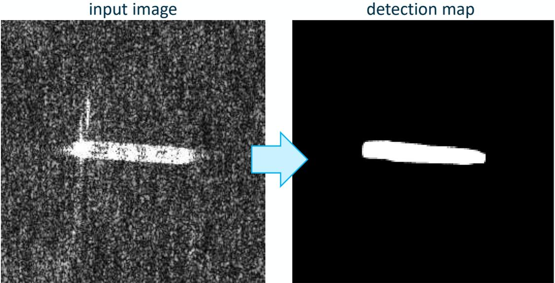
The threshold changes adaptively and the detector is usually applied on pixel-bases. 30 x 50 km<sup>2</sup> VHR SAR image @1.5m pixel spacing is ~660 \* 10<sup>6</sup> pixels
