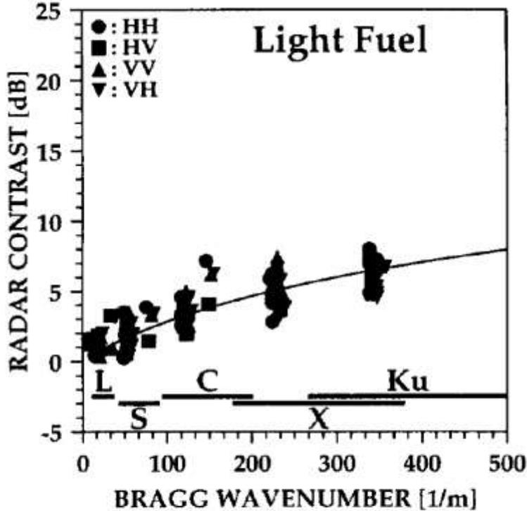
Figure 1: Radar contrast induced by the light fuel MARPOL spills as a function of the Bragg wavenumber  $k_B$ . The bars indicate how the Bragg wavenumbers are covered by the different radar bands. The solid line is computed from *Marangoni* wave damping theory [9]. © V. Wismann, 1993
