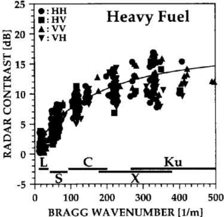
Figure 2: Same as Fig. 1, but for the heavy fuel spills. © V. Wismann, 1993
