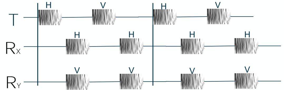
Quad-pol: 4 combinations  $[\dot{S}_{hh}, \dot{S}_{hv}, \dot{S}_{vh}, \dot{S}_{vv}] \longrightarrow$  Doubling of the PRF
