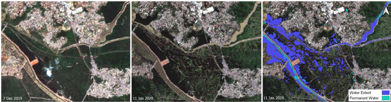
Figure 15: QC approach for the flood extent product. Reference image to the left, source imagery used for mapping in the middle and flood map to the right
