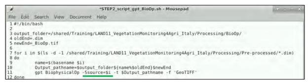
On lines **3 to 5** we specify input parameters, such as the path to out output directory and the input file end and output file end, respectively. Our output format will be GeoTIFF, therefore the output file end must reflect this.
