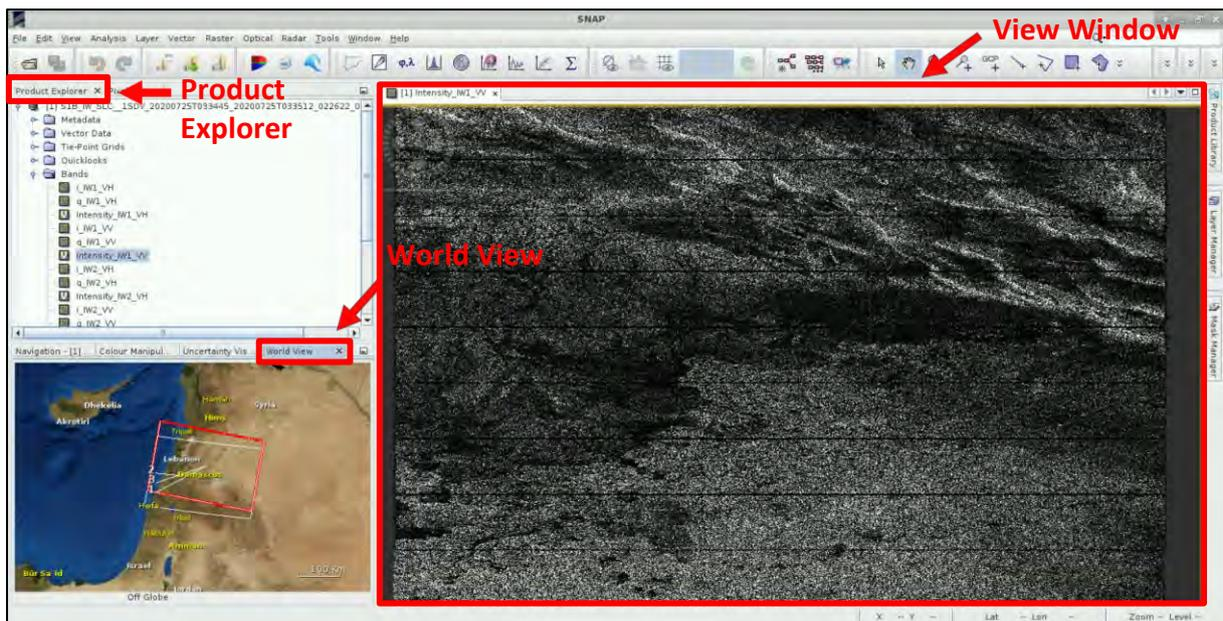
Open the **Intensity\_IW2\_VV** and **Intensity\_IW3\_VV** bands as well, and go to **Window** → **Tile Horizontally**. Go to the **Navigation** tab and click on the two icons shown within the red rectangular below, to synchronize the views and the cursor position between the views. (See NOTE 3).
