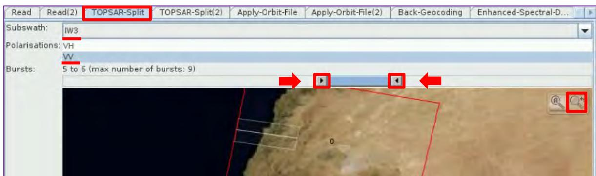
In the **TOPSAR-Split(2)** tab **Zoom in** to the product and select: **Subswath: IW3, Polarisations: VV, Bursts: 3 to 4** (drag the two sliders accordingly).
