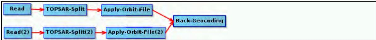
In the **Back-Geocoding** tab set: **Digital Elevation Model: SRTM 1Sec HGT (Auto Download)**, select the **“Output Deramp and Demod Phase”** option as well and leave the rest parameters as by default.
