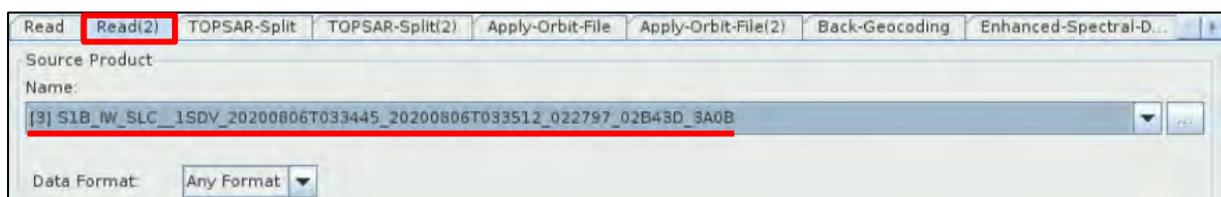
In the **TOPSAR-Split** tab **Zoom in** to the product and select: **Subswath:** IW3, **Polarisations:** VV, **Bursts:** 3 to 4 (drag the two sliders accordingly).
