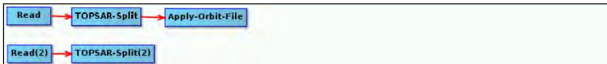
Repeat the same to add the **Apply-Orbit-File(2)** operator and connect it with the **TOPSAR-Split(2)** operator.
