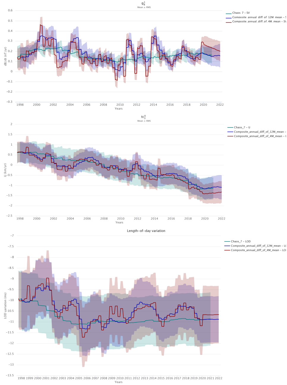
Figure 5.2: Re-analyses of the core-surface flow and magnetic field from 1998 to 2020, using several datasets: CHAOS-7 Gauss coefficients (cyan), 4-monthly GVO data (red) and annual means of 4-monthly GVO data (blue). top: SV coefficient g_8^1 ; middle: flow coefficient t_3^0 ; bottom: associated length-of-day (LOD) variations.
