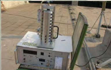
Quartz Crystal Micro balance (QCM) Cascade Impactor
