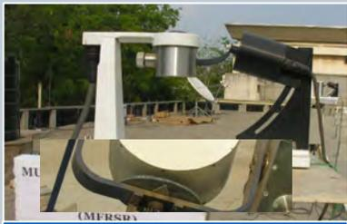
Multi-Filter Rotating Shadow-Band Radiometer (MFRSR)
