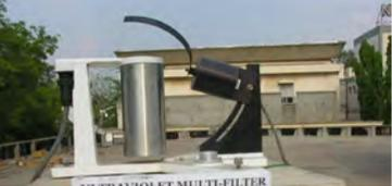
UV Multi-Filter Rotating Shadow Band Radiometer
