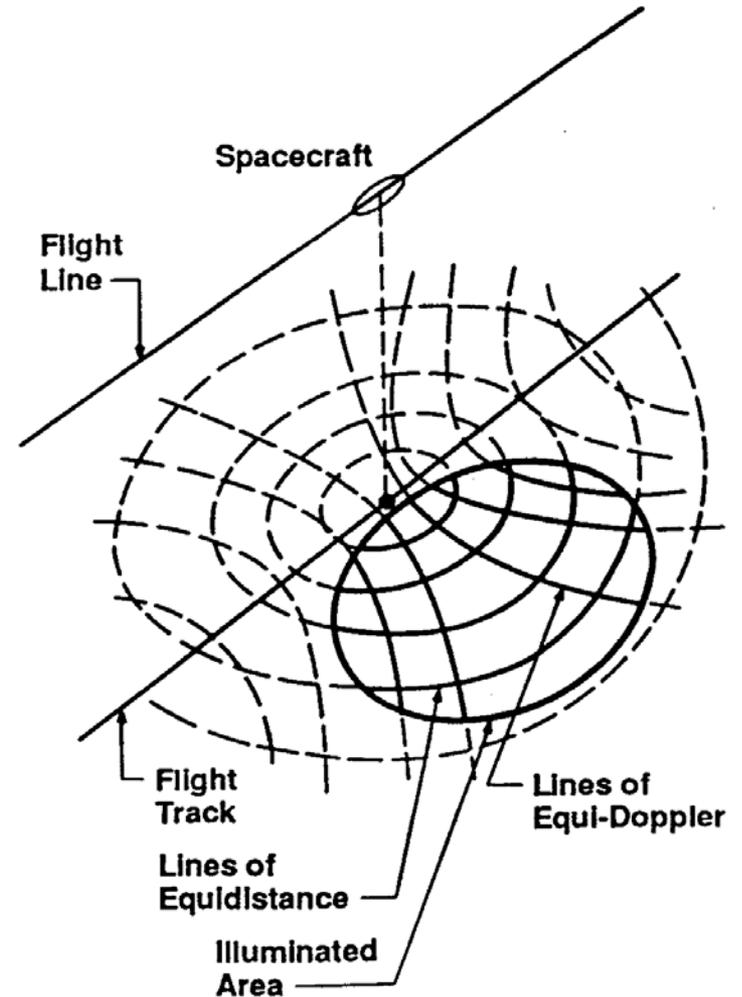
A SAR makes use of measurements of the range and Doppler shift of the radar returns to locate ground points. The signals from many returns are analysed together to image ground elements  $\sim 5 \times 20\text{m}$  in size, much smaller than would be possible with a stationary antenna of the same size - hence the Synthetic Aperture.
