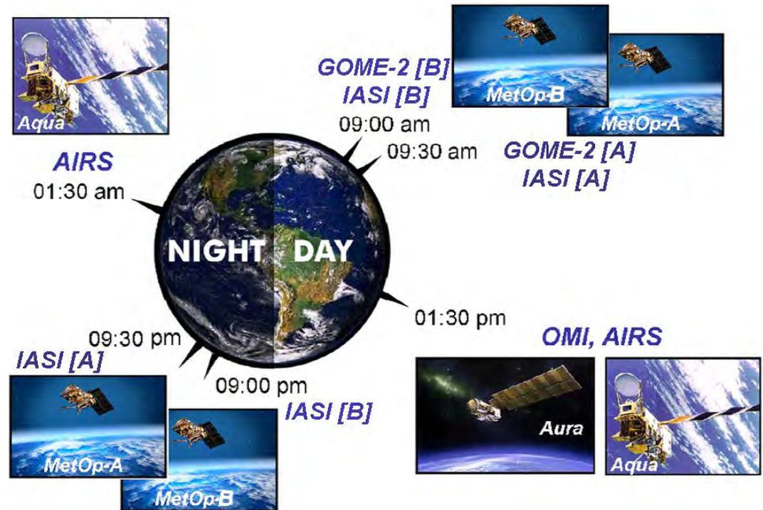
Constellation of 6 satellite hyperspectral sensors used to monitor volcanoes
