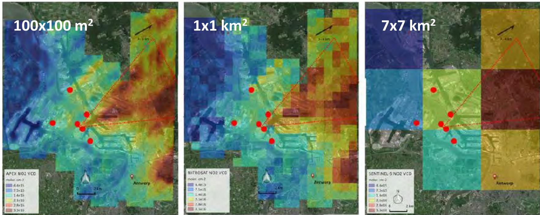
Airborne APEX hyperspectral NO<sub>2</sub> columns measured over Antwerp (Courtesy F. Tack). Native resolution is approximately 100x100 m<sup>2</sup>. Main sources can still be detected at 1x1 km<sup>2</sup>.
