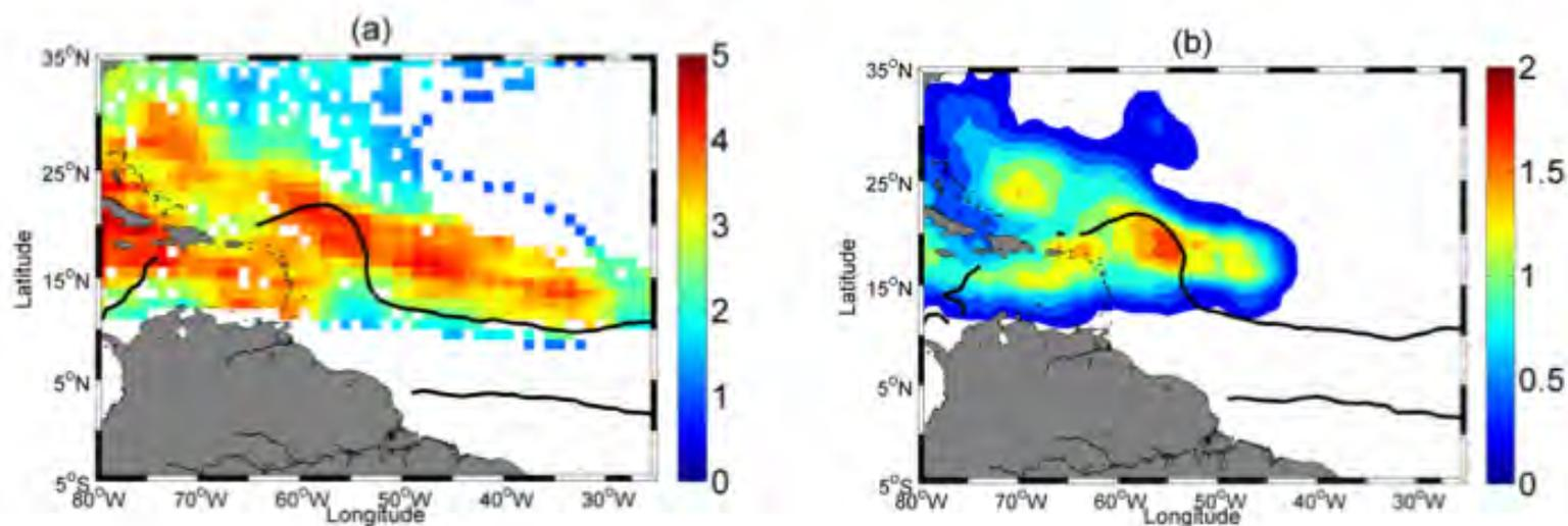
FIG.2 The number of 1950 through 2010 “best track” TC per one degree square (smoothed by a 3° x 3° block average) (a) that evolves as Cat 4-5 somewhere along their path and (b) that intensified locally to Cat 4-5. The black curve is showing the historical extent of the Amazon-Orinoco river plume during the hurricane peak season (August to October).
