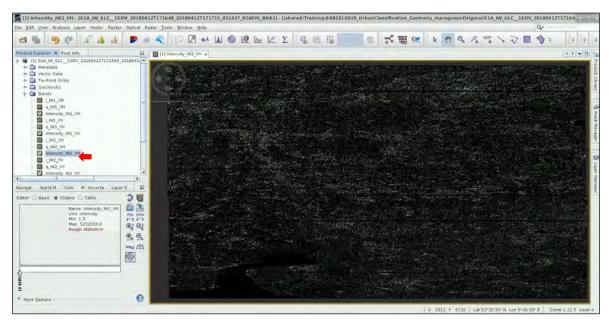
NOTE 4: The Interferometric Wide (IW) swath mode captures three sub-swaths using Terrain Observation with Progressive Scans SAR (TOPSAR). Each sub-swath image consists of a series of bursts. The input product contains 3 IW bands, and 8 bursts. Mexico City is located on the IW3 sub-swath of the
