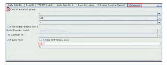
NOTE 7: Coherence is the fixed relationship between waves in a beam of electromagnetic (EM) radiation. Two wave trains of EM radiation are coherent when they are in phase. That is, they vibrate in unison. In terms of the application to things like RADAR, the term coherence is also used to describe systems that preserve the phase of the received signal.
