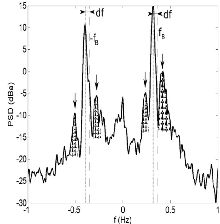
Two prominent peaks due to waves (approaching and receding). Shift from linear wave frequency is due to surface current component in the direction of the antenna
