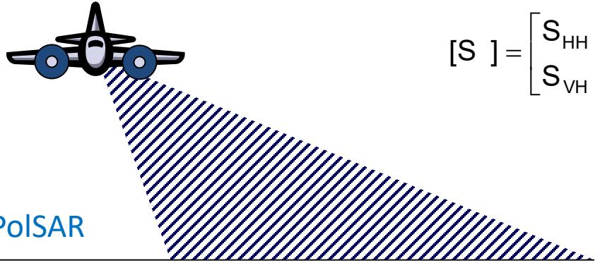
$$[S] = \begin{bmatrix} S_{HH} & S_{HV} \\ S_{VH} & S_{VV} \end{bmatrix}$$
