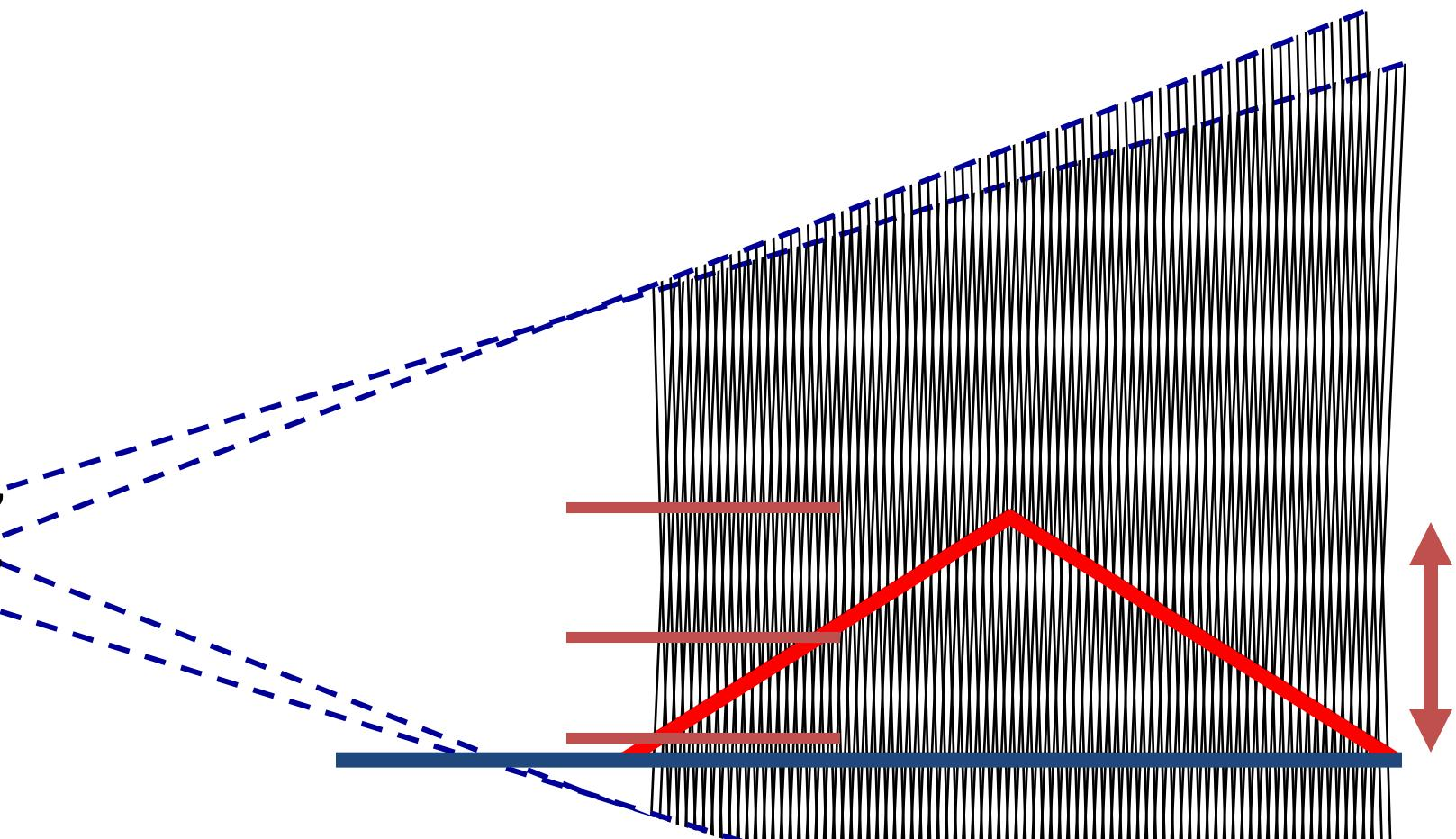
The Phase-to-Height Sensitivity increases with increasing the spatial baseline (i.e.  $\Delta\theta$  or  $B\bar{r}$ );
