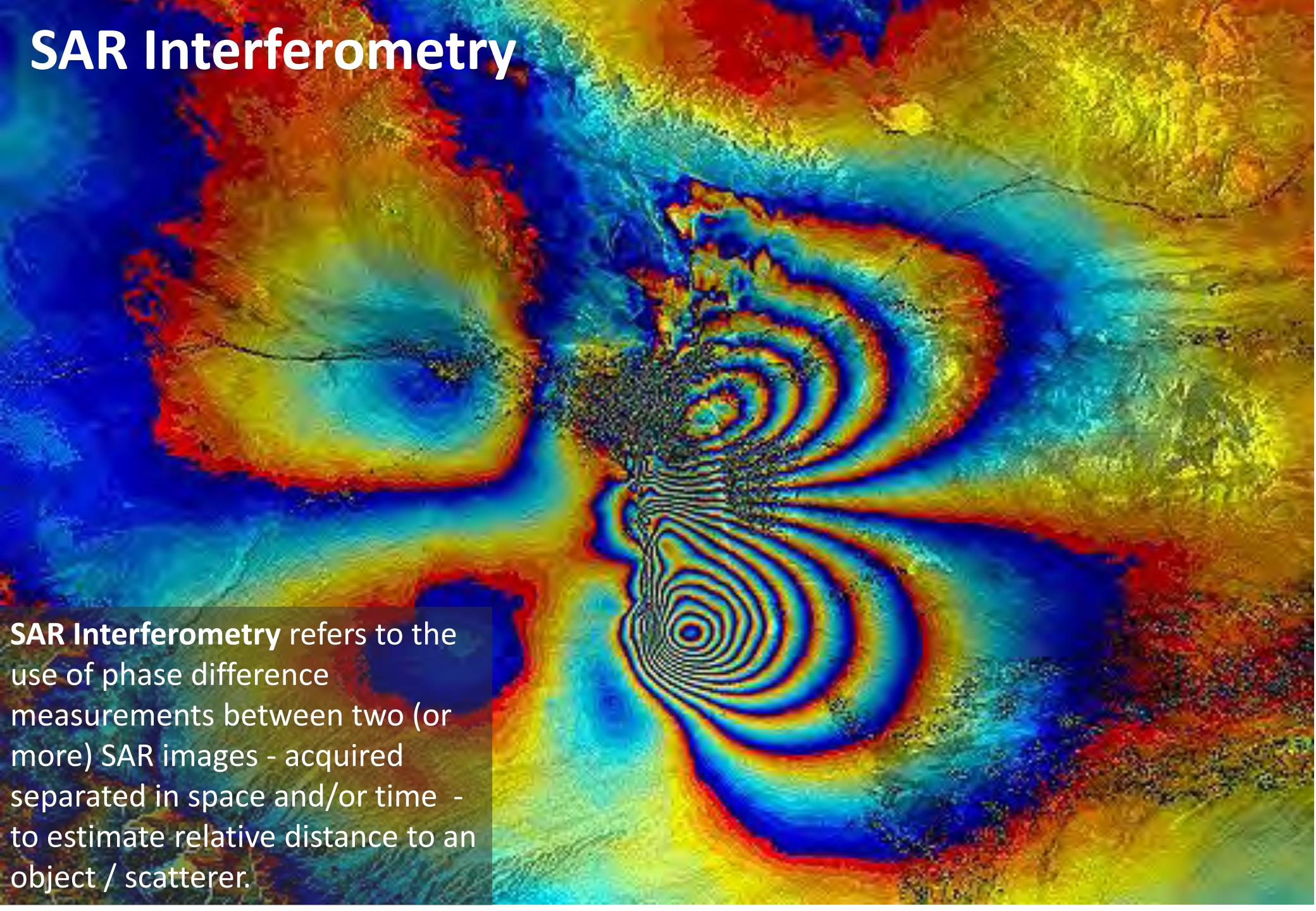
**SAR Interferometry** refers to the use of phase difference measurements between two (or more) SAR images - acquired separated in space and/or time - to estimate relative distance to an object / scatterer.
