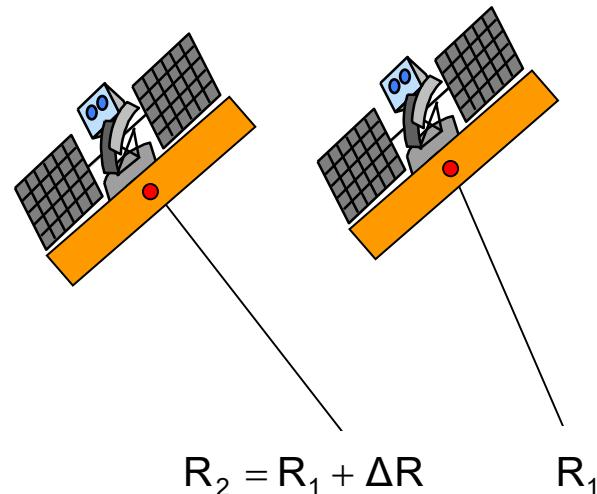
Signal from resolution cell P in Image 1:  $i_1 = |i_1| \exp[-i(2\frac{2\pi}{\lambda}R_1) + \varphi_{s1}]$
