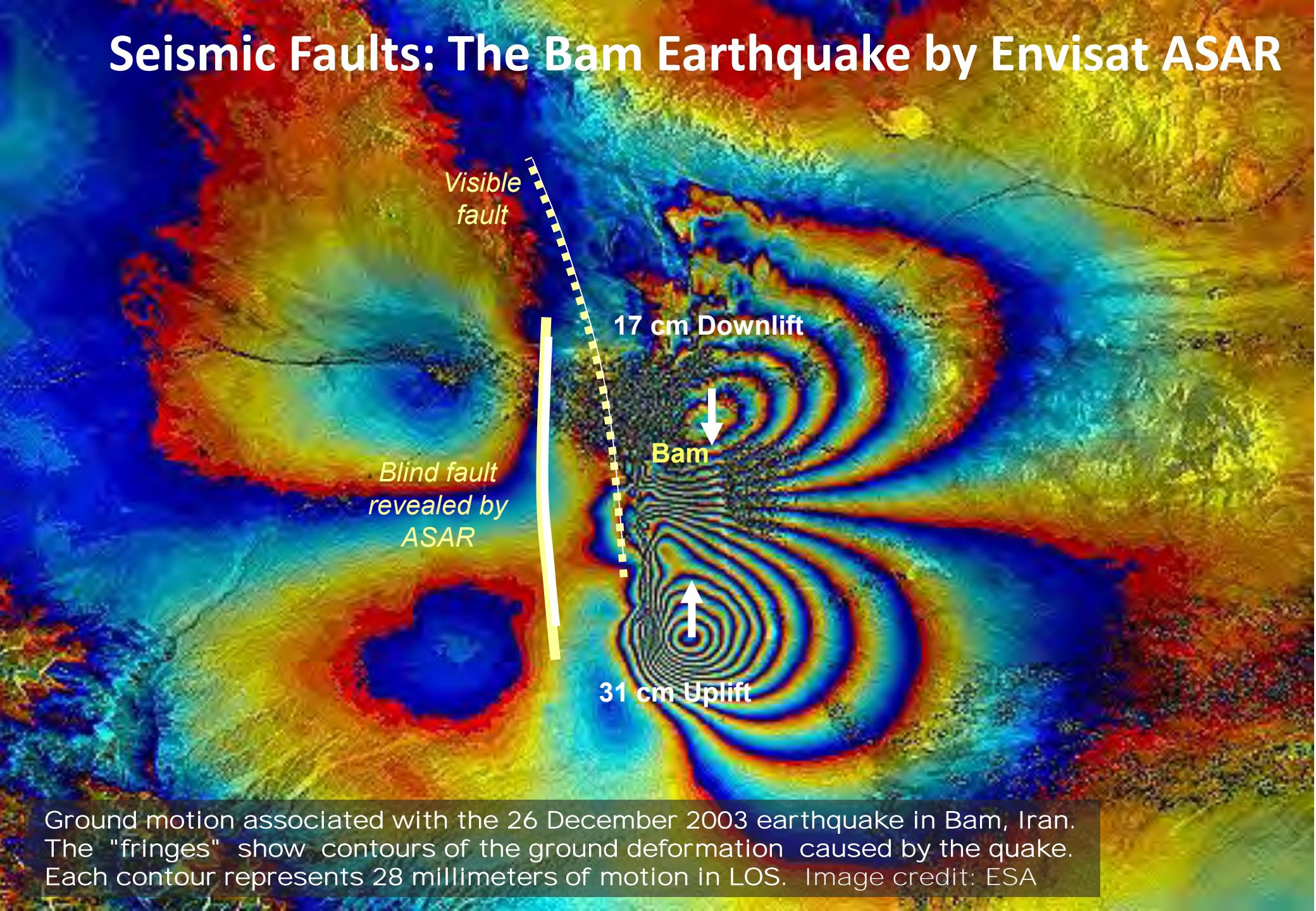
Ground motion associated with the 26 December 2003 earthquake in Bam, Iran. The "fringes" show contours of the ground deformation caused by the quake. Each contour represents 28 millimeters of motion in LOS. Image credit: ESA
