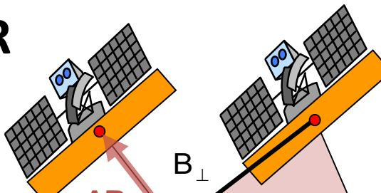
Example ERS: Space-borne C-band ( $\lambda=0.056\text{m}$ ) interferometer with incidence  $\theta=23^\circ$  at range  $R=870\text{km}$
