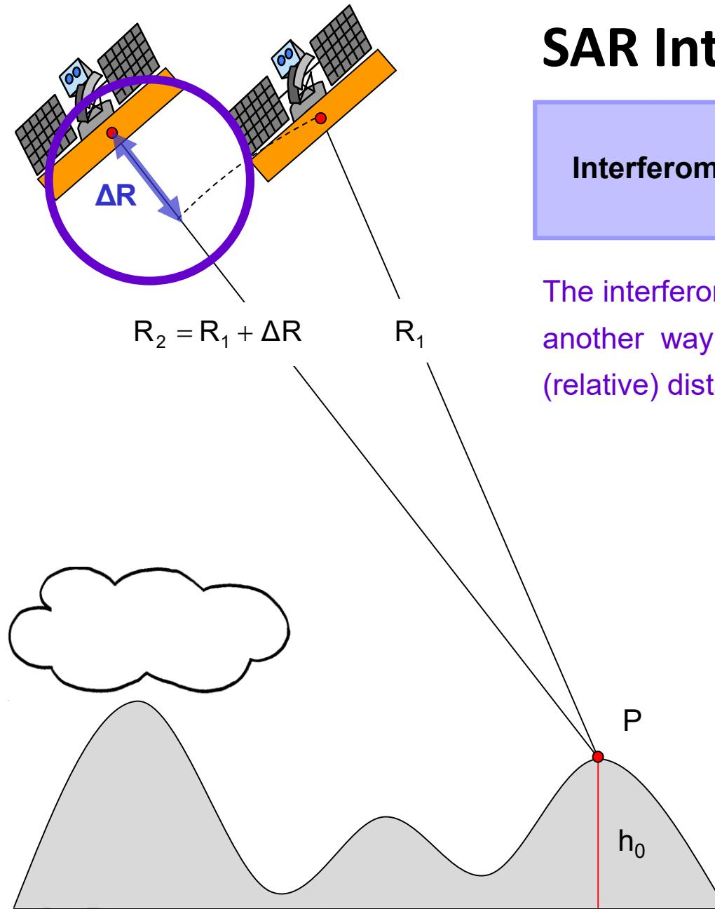
$$\text{Interferometric Phase: } \varphi = 2\frac{2\pi}{\lambda} \boxed{\Delta R}$$
