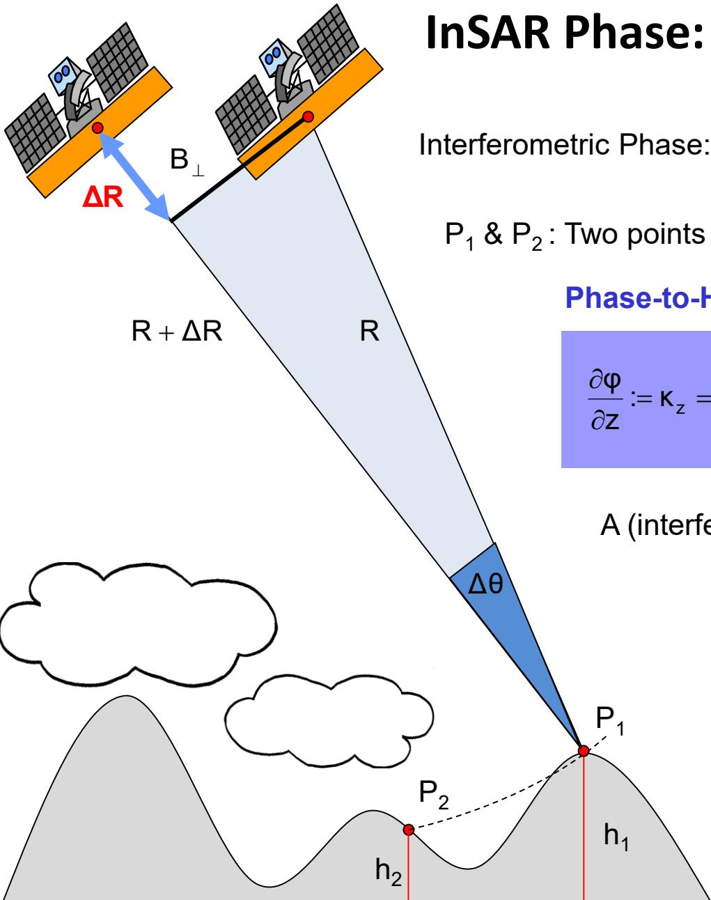
Interferometric Phase:  $\varphi = 2\frac{2\pi}{\lambda}\Delta R + 2\pi N$  where  $N = 0, \pm 1, \pm 2$
