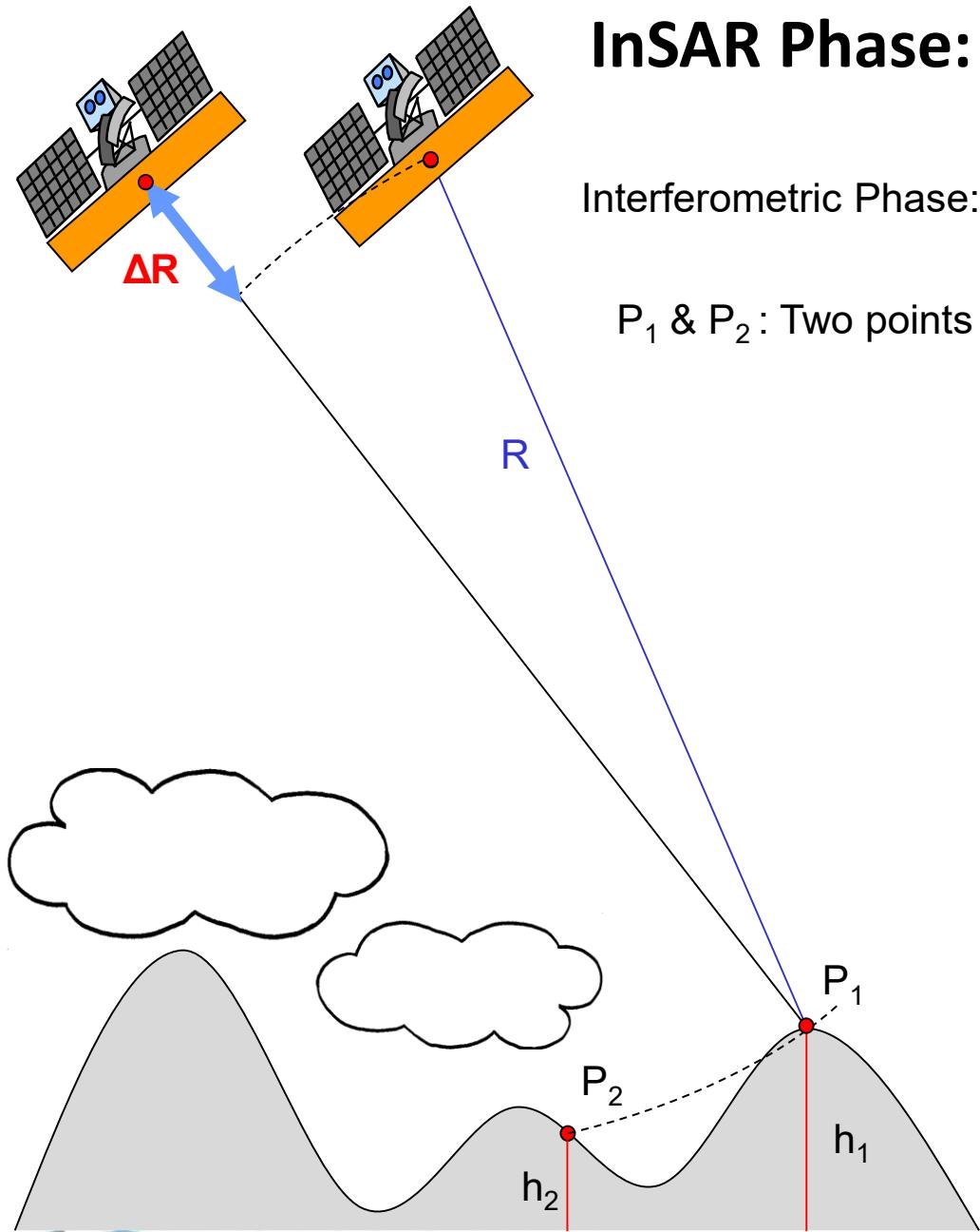
$$\text{Interferometric Phase: } \varphi = 2\frac{2\pi}{\lambda} \Delta R + 2\pi N \quad \text{where} \quad N = 0, \pm 1, \pm 2$$
