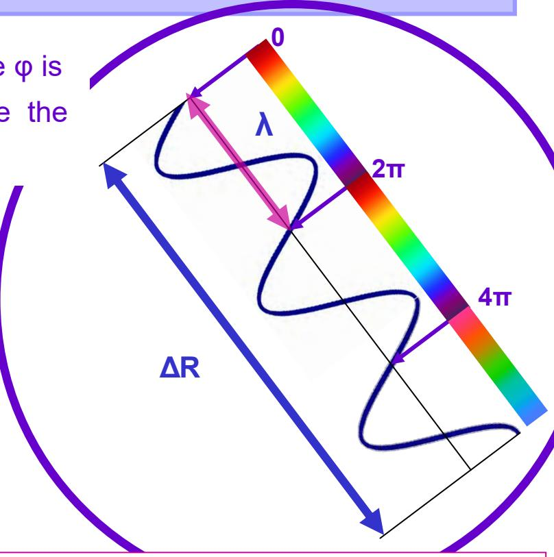
Phase measurements in interferometric systems can be made with a degree level accuracy. At radar wavelengths of 1-90cm (Ku to P-band) this corresponds to millimeter accuracy !!!
