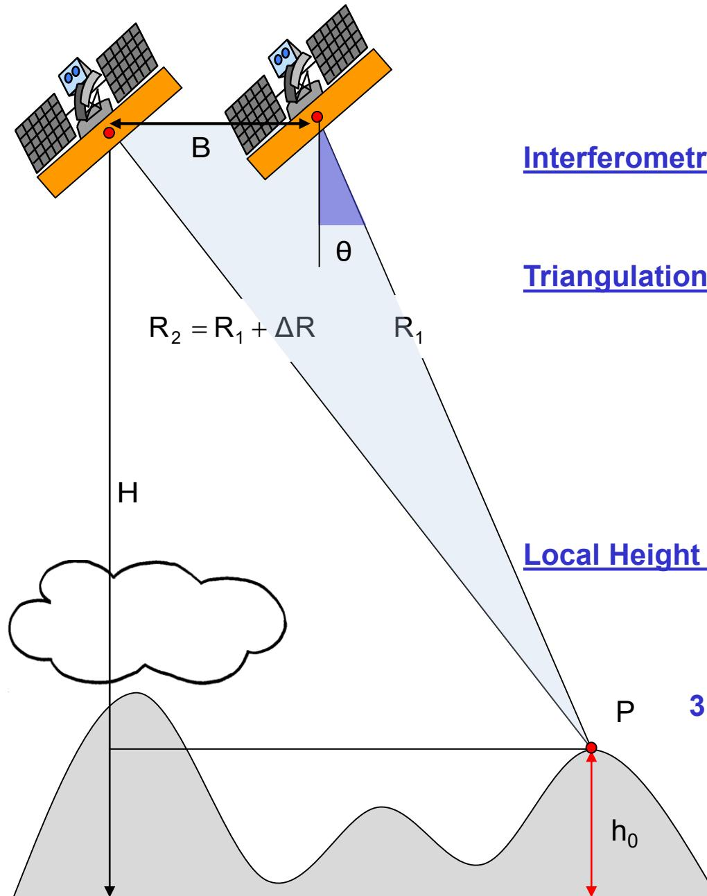
Interferometric Phase (1):  $\varphi = 2\frac{2\pi}{\lambda} \Delta R + 2\pi N \quad N = 0, \pm 1, \pm 2$
