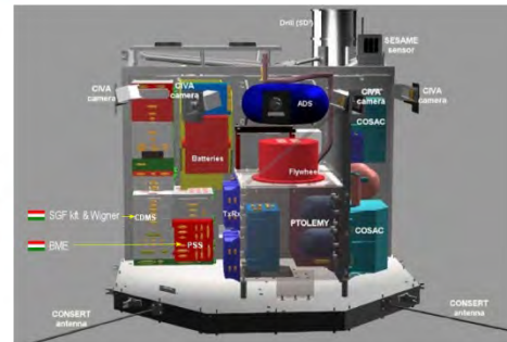
Hungarian contributions to the core system parts of Philae: Central Computer and Power System
