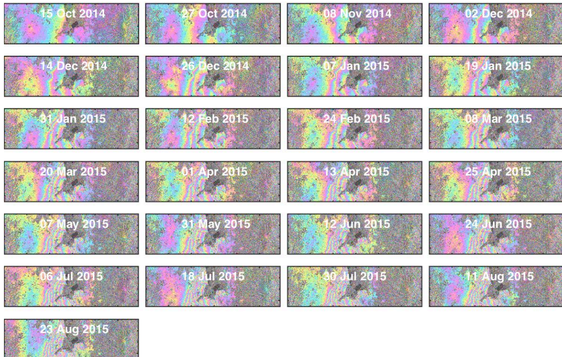
Figure 1. Single master interferograms (20 looks in range, 4 looks in azimuth). The master data is 3 Oct 2014.
