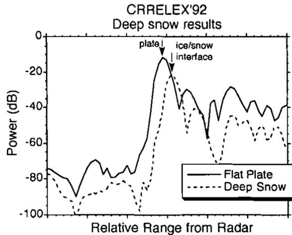
Figure 13. Comparison of  $K_u$ -band radar returns at  $0^\circ$  incidence angle from a 21-cm snow pile and a metal plate on top of the snow pile. The ice thickness was 12 cm. This demonstrates that the return from snow-covered saline ice is dominated by scattering from the snow-ice interface.
