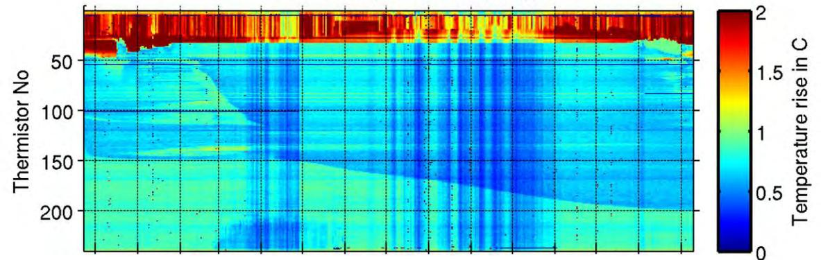
Sea ice temperatur and thermal conductivity measured by thermistorstring with heating function
