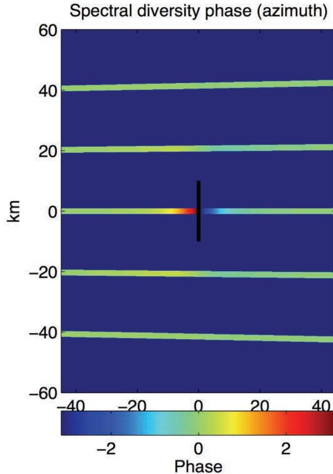
~1.7 m azimuth displacement for one phase cycle
