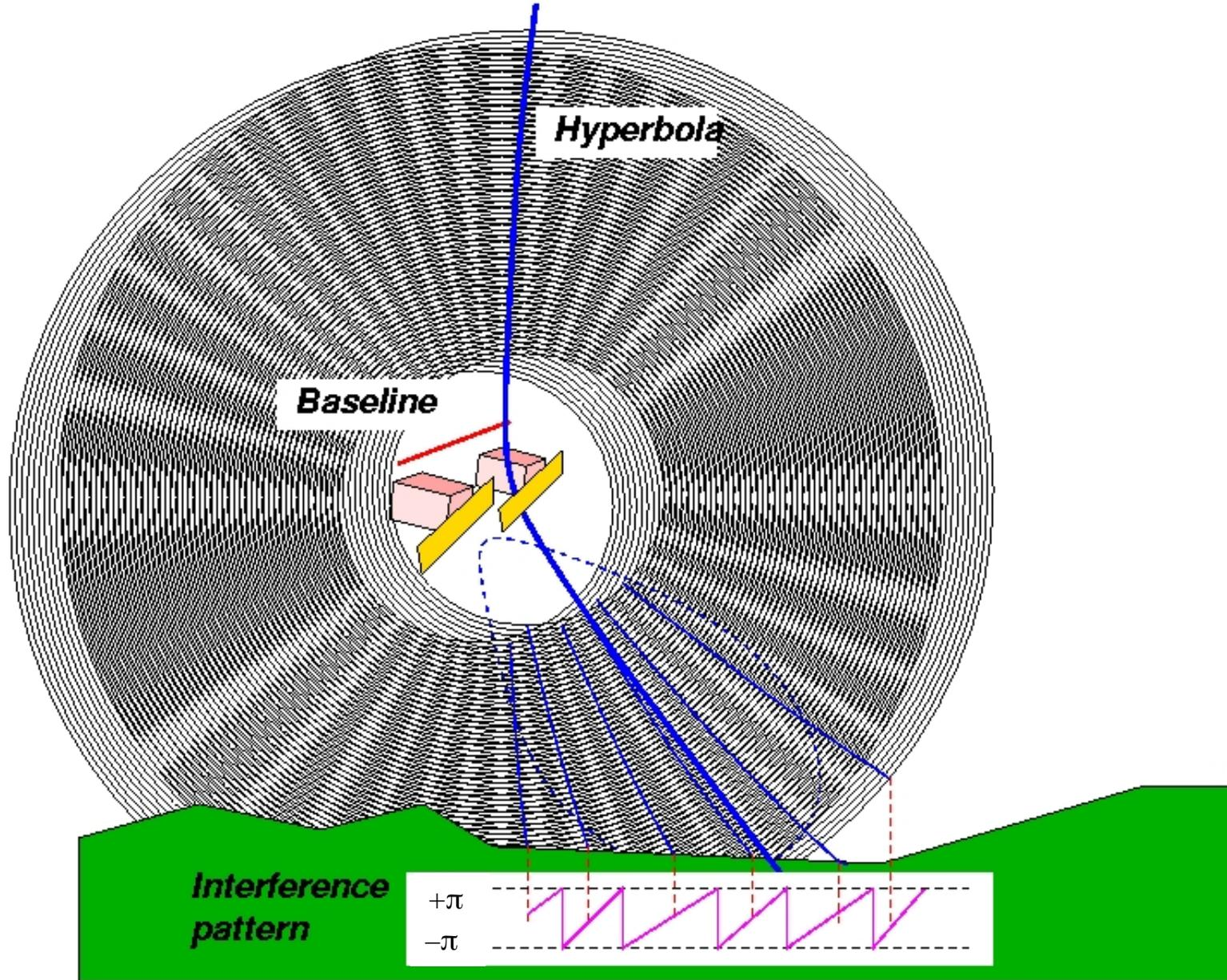
Interference phase at ground depends mainly on horizontal position, but also a little on the vertical position
