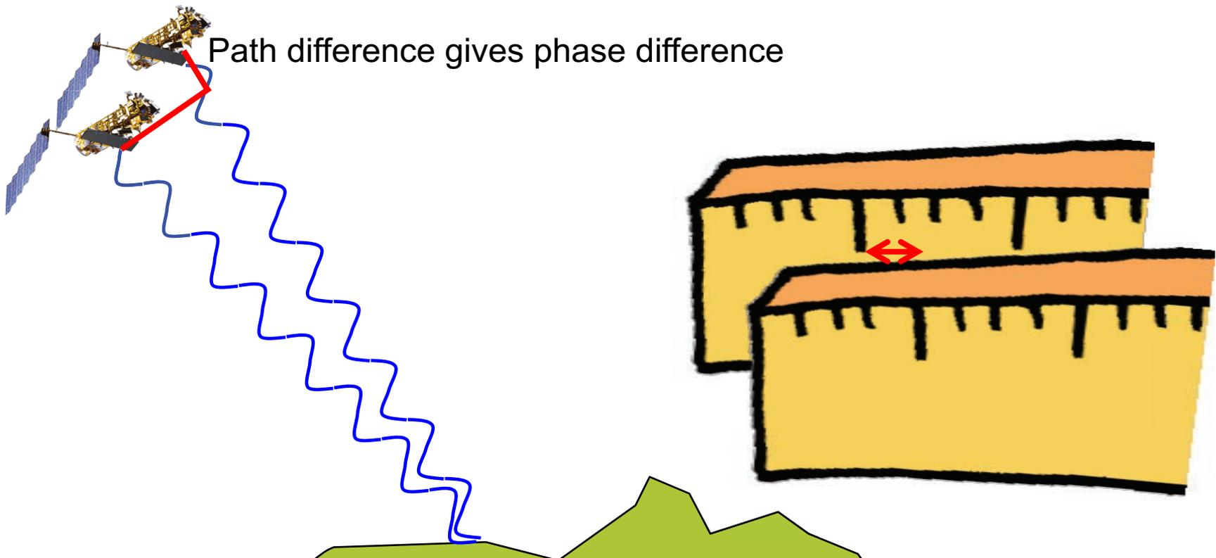
Interferometric phase is phase difference
