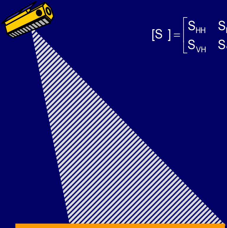
$$[S] = \begin{bmatrix} S_{HH} & S_{HV} \\ S_{VH} & S_{VV} \end{bmatrix}$$
