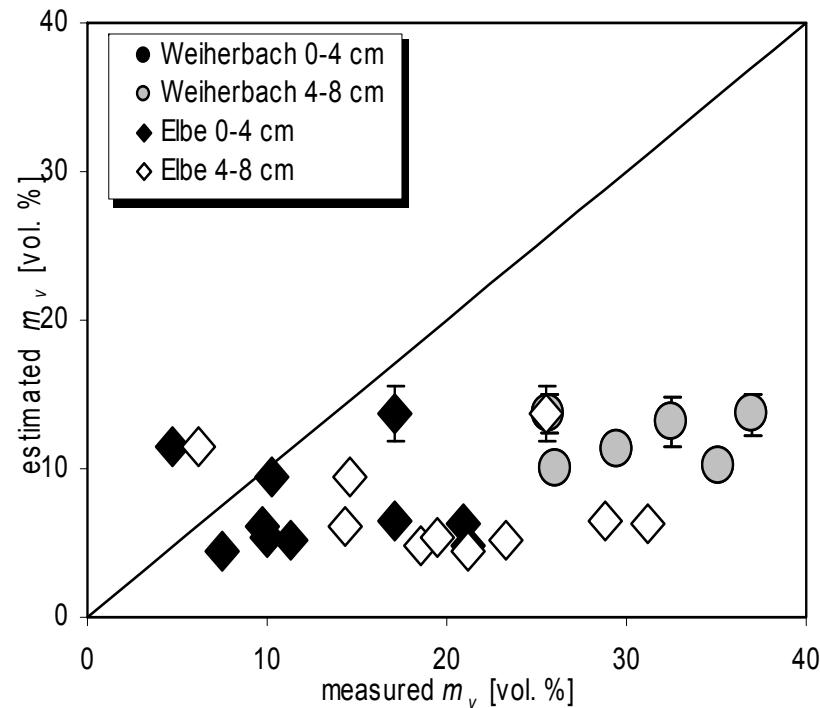
Measured versus estimated volumetric moisture content  $m_v$  [vol. %] using SPM
