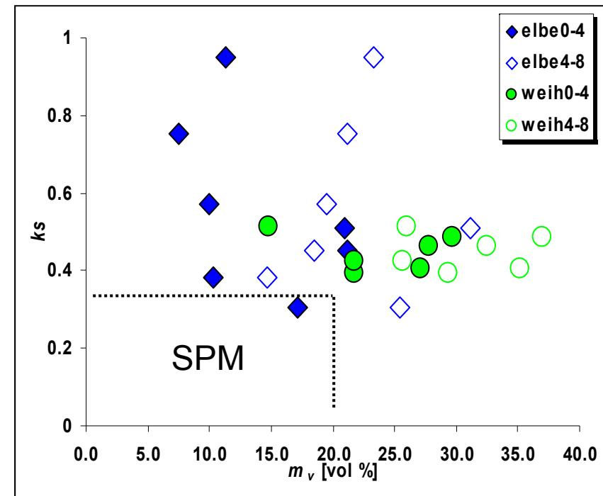
Validity range of the SPM for the ground measurements - surface roughness against volumetric soil moisture
