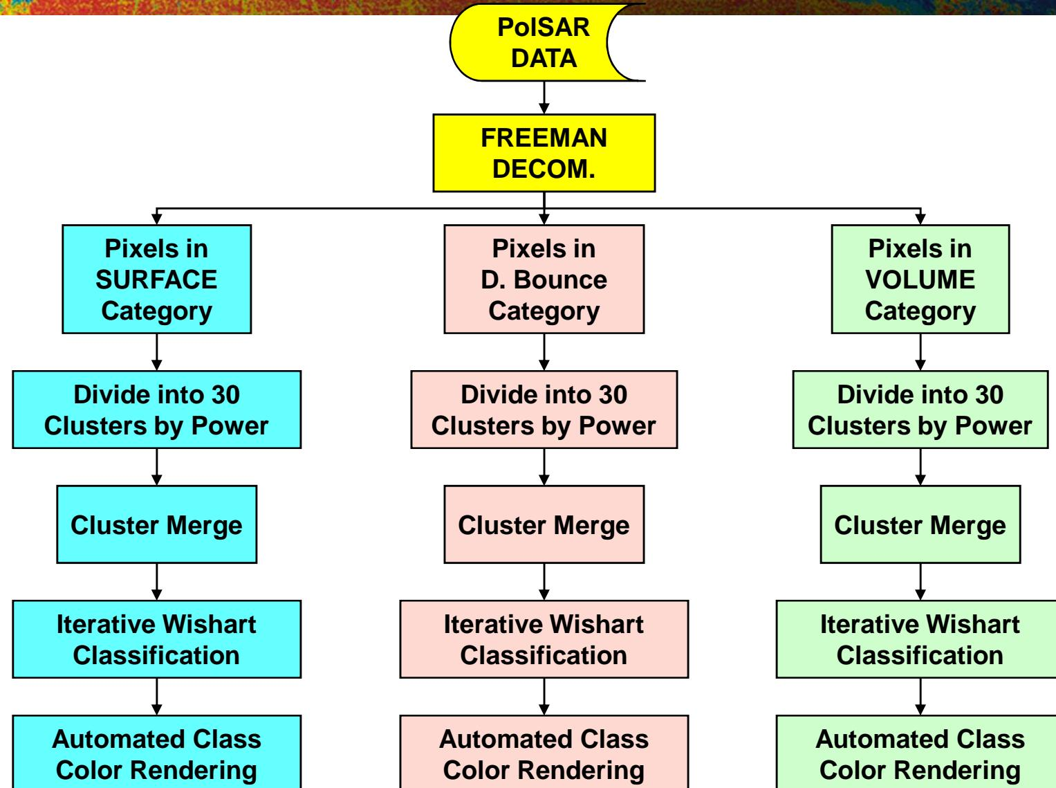
$$\text{Cluster Merging } D_{ij} = \frac{1}{2} \{ \ln(|V_i|) + \ln(|V_j|) + \text{Tr}(V_i^{-1}V_j + V_j^{-1}V_i) \}$$
