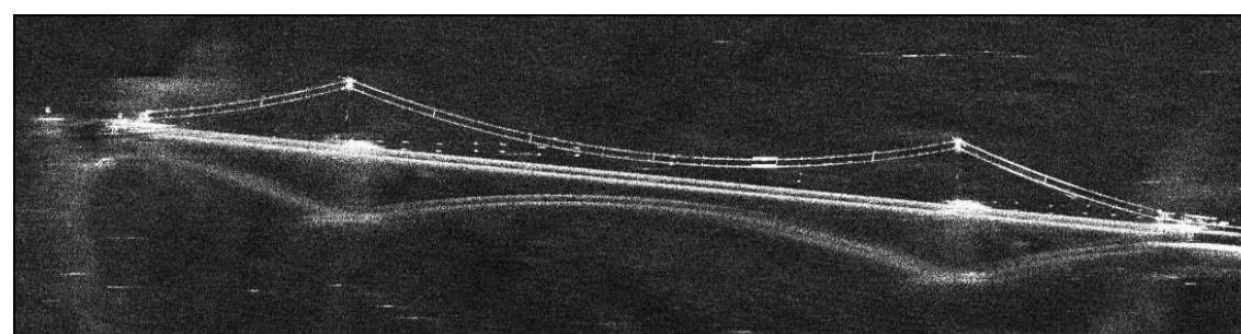
EMISAR C-Band Polarimetric SAR Image of StoreBelt Bridge
