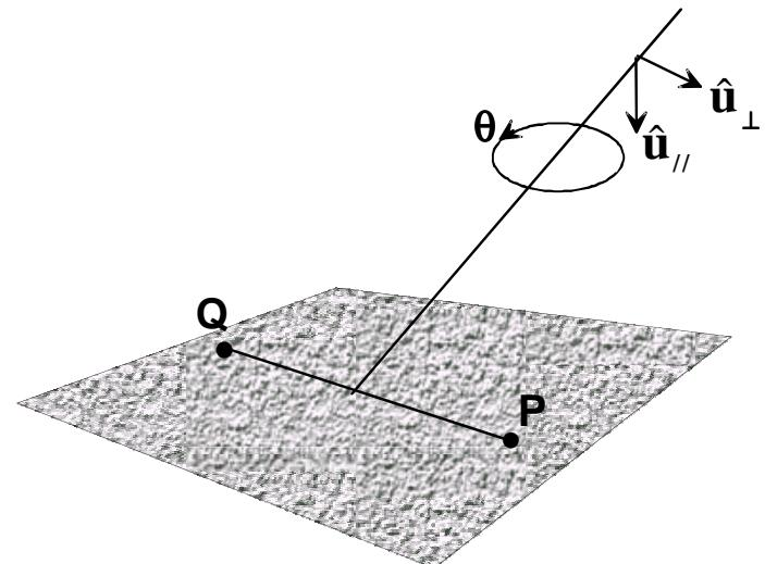
$$\langle [T(\theta)] \rangle = [R_3(\theta)] \langle [T] \rangle [R_3(\theta)]^{-1}$$
