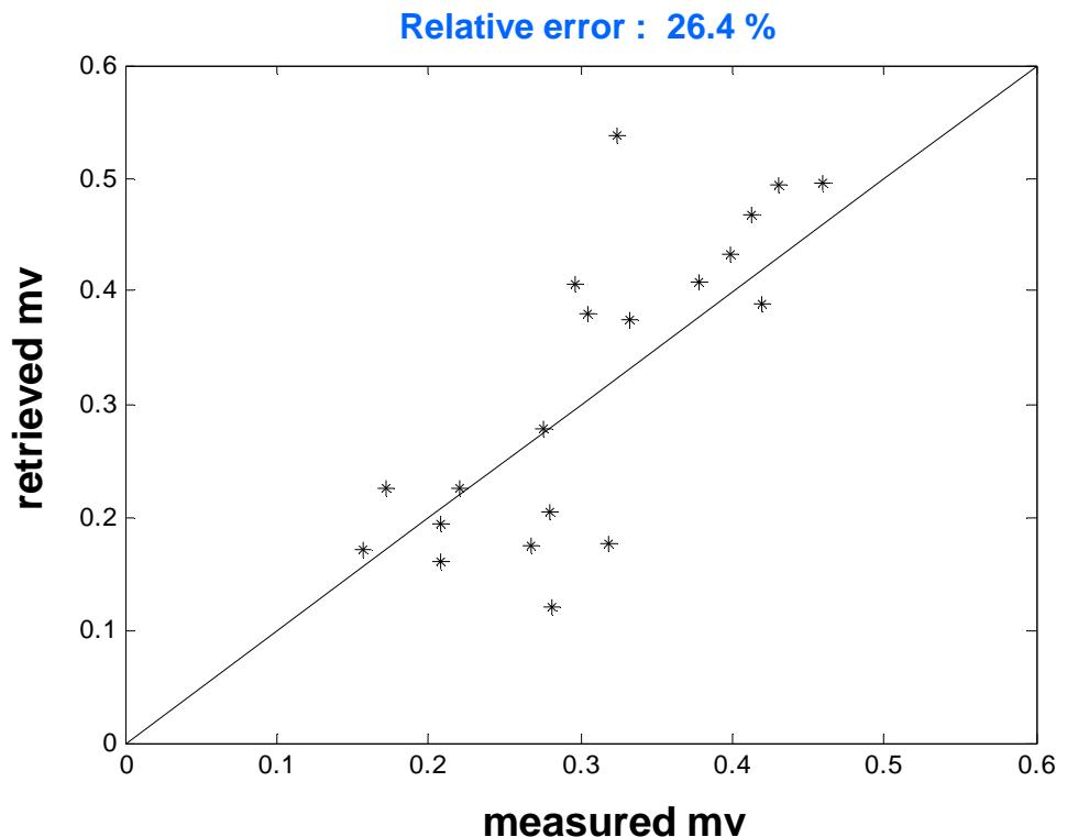
$$\text{relative error} = \left| \frac{\text{retrieved mv} - \text{measured mv}}{\text{retrieved mv}} \right| \cdot 100$$
