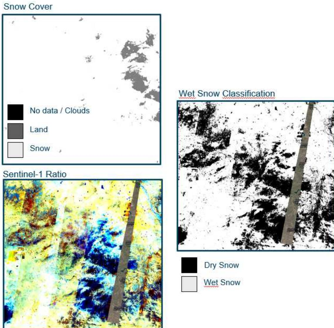
Figure 12 The wet snow classification (right) is derived from Sentinel-1 backscatter ratio (lower left) combined with the snow cover maps (upper left). The artefact in the snow classification results from missing Sentinel-1 data. Note that the land mask was not applied in this example.
