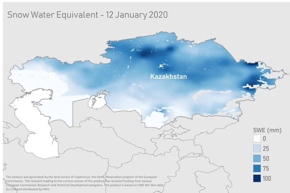
*Figure 13. Copernicus Snow Water Equivalent (SWE) as of 12 January 2020. SWE describes the equivalent amount of liquid water stored in the snowpack, which indicates the water column that would theoretically result should the whole snowpack melt instantaneously. Source: Copernicus Global Land Service.*
