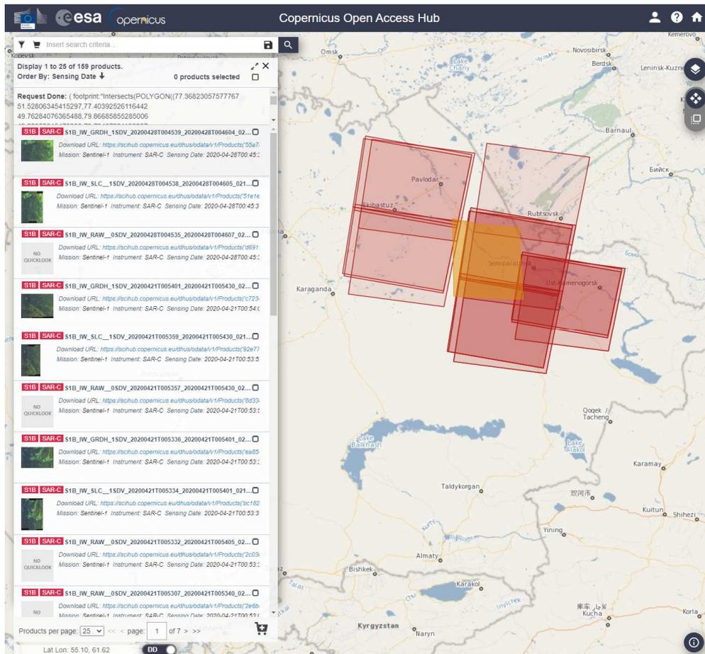
Figure 17 Sentinel-1 coverage in red and AOI in orange. Well visible is the gap in coverage.
