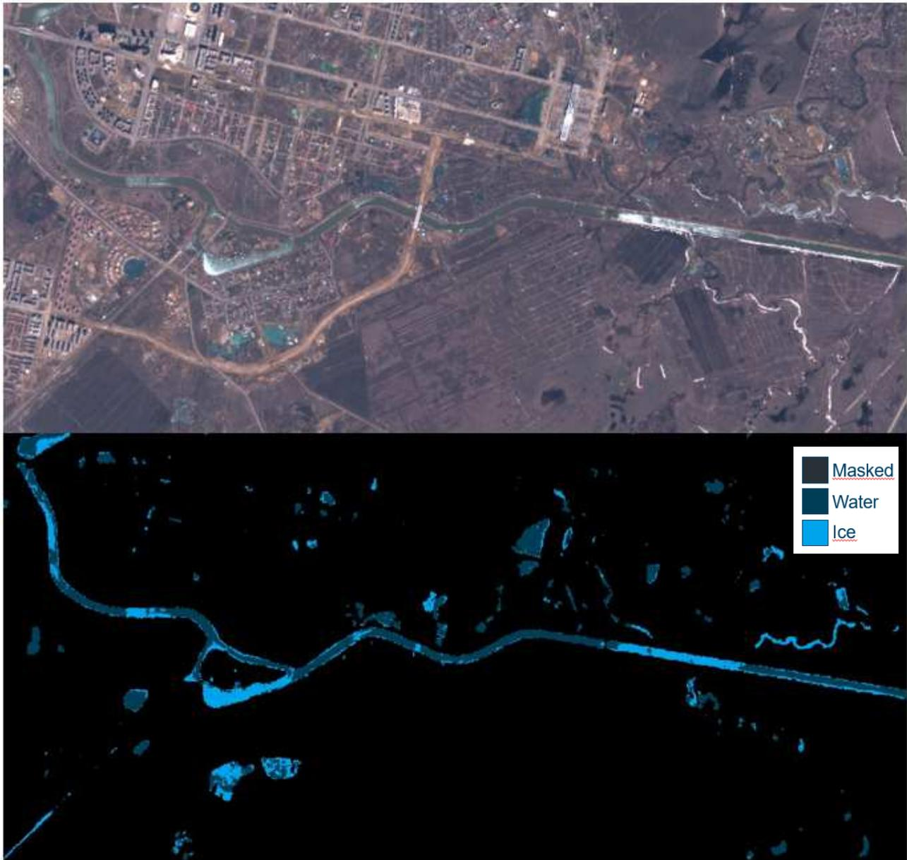
Figure 23. Example of ice jam detection in Nur-Sultan using Sentinel-2 imagery acquired on April 11, 2019.
