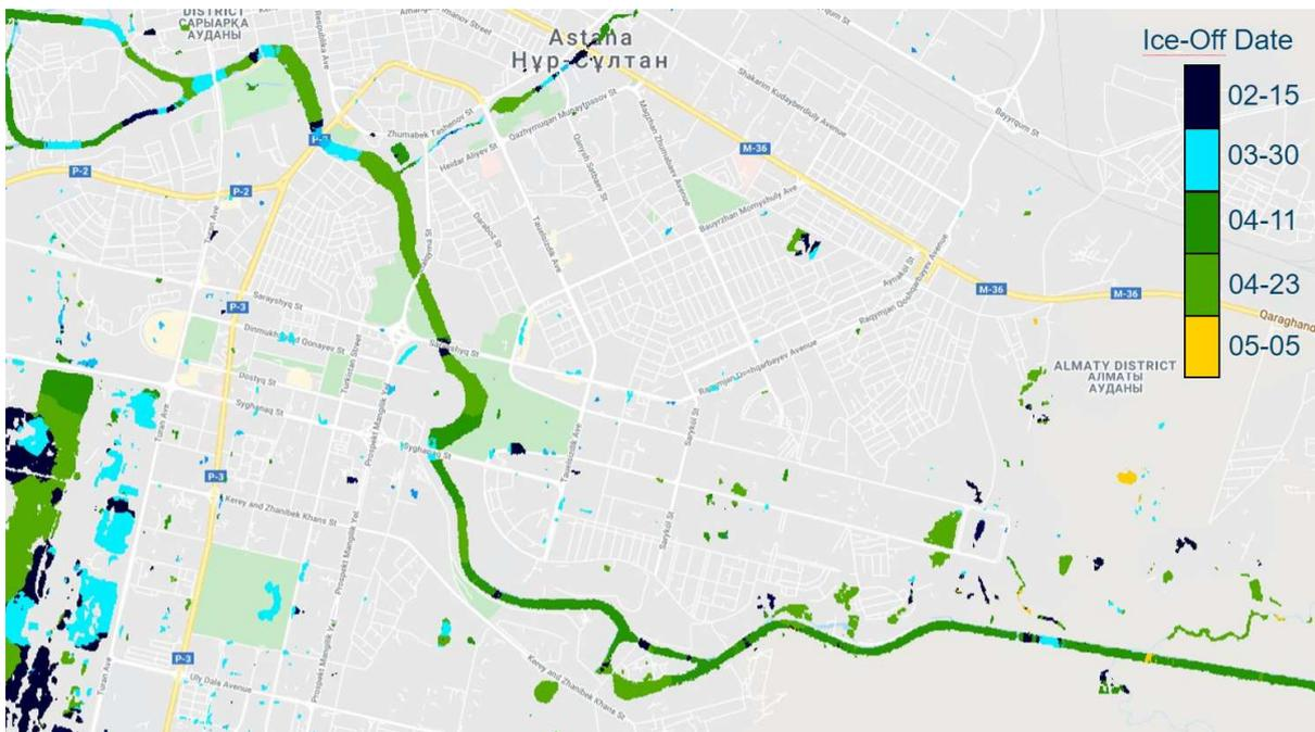
Figure 19 Ice break-up sequence of Ishim River in Nur-Sultan in Spring 2018. Analysis is based on Sentinel-1 change detection.
