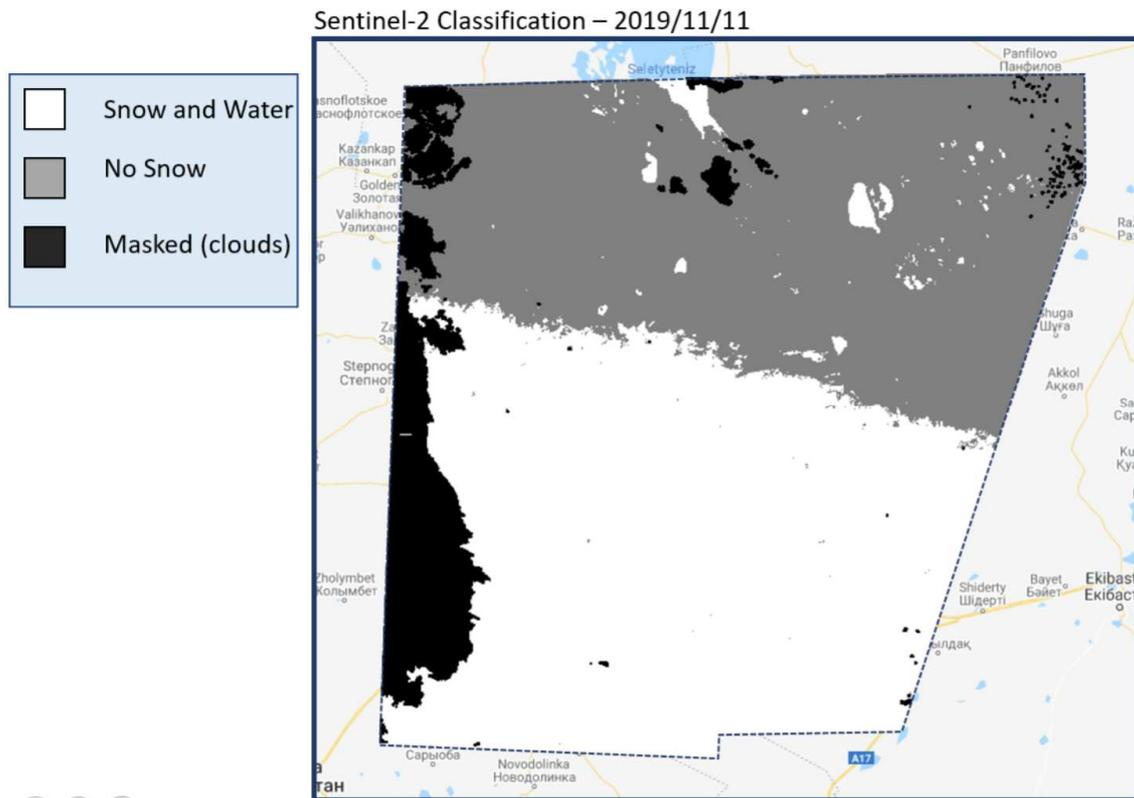
Figure 7. From raw Sentinel 2 data (upper left), to NDSI (upper right) and the final categorical map with snow/water (ice), no snow and cloud classes. In addition to this, in the final product the clouded areas will be filled with Sentinel 3, MODIS and SAR data. The water areas will be masked with the detailed surface water mask from project EOC003.
