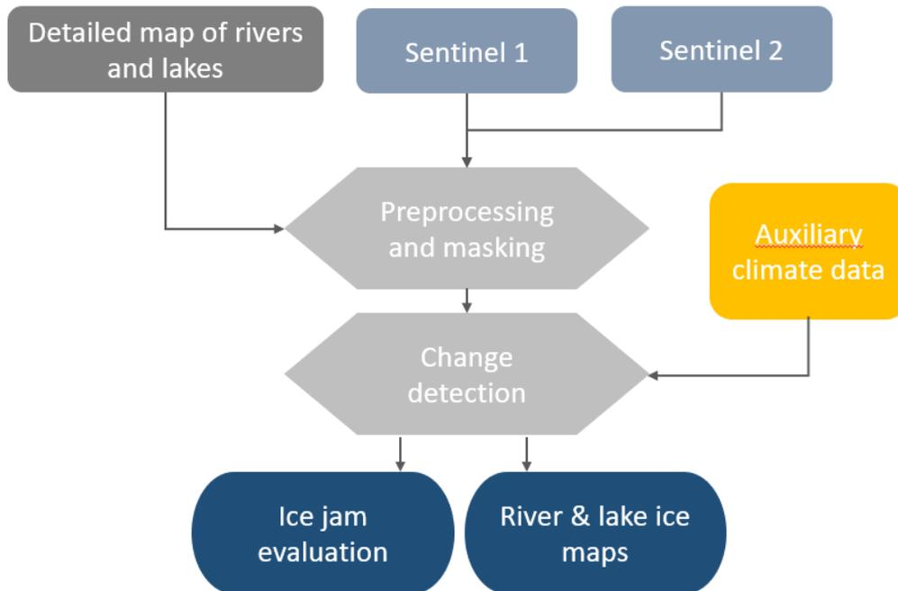
Figure 20 Workflow for river and lake ice dynamics monitoring as provided under service 2. The detailed map of rivers and lakes was taken from a previous technical assistance (EOC0003).
