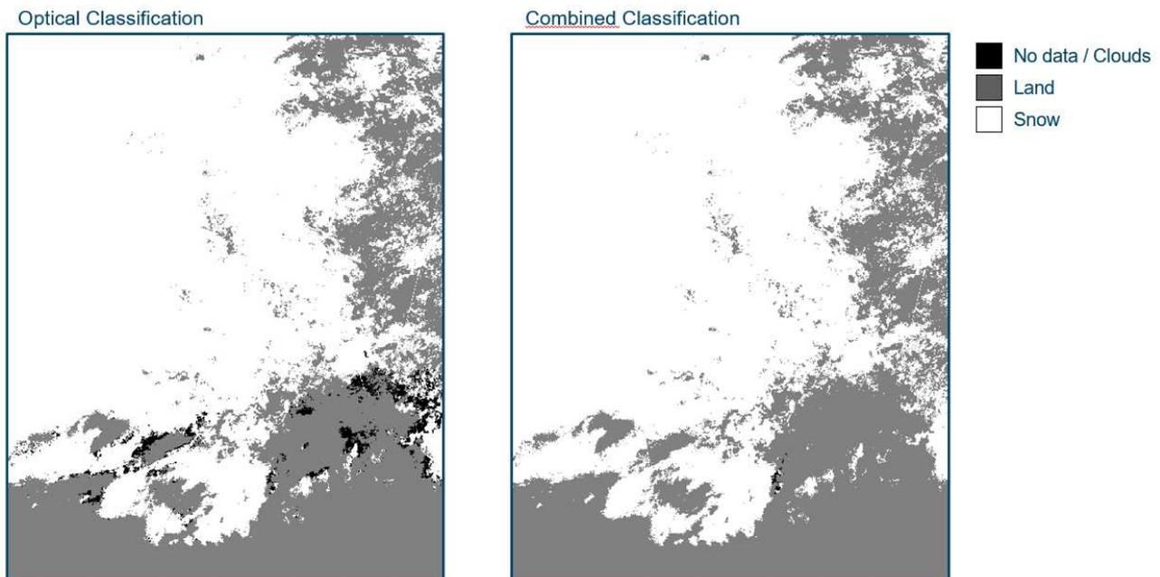
Figure 10. Example of gap filling of the optical results using Sentinel-1 data, resulting in very little no-data in the final combined results.
