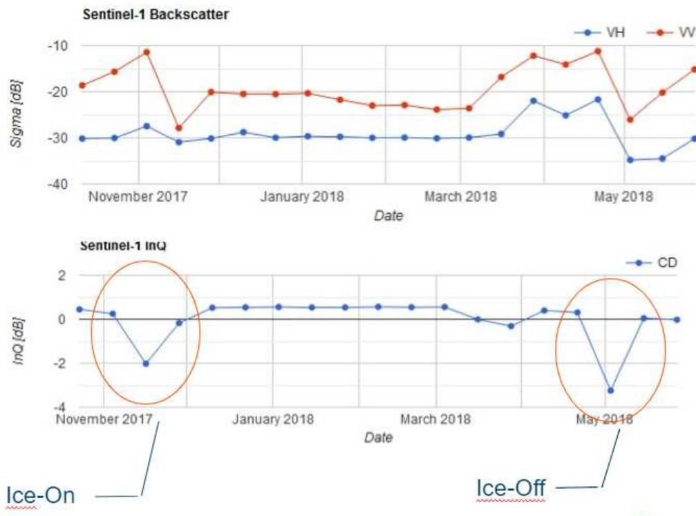
Figure 22 Backscatter signal from Sentinel-1 used to detect ice on and ice off periods on water. The approach is based on Nielsen et al (2017).
