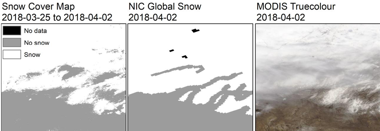
Figure 15 Comparison between one of the new Snow Cover maps (left), a NIC Global Snow Cover map from the same area (centre), and a MODIS True Colour Composite. Clearly visible is the added spatial detail of the new map produced under this project.
