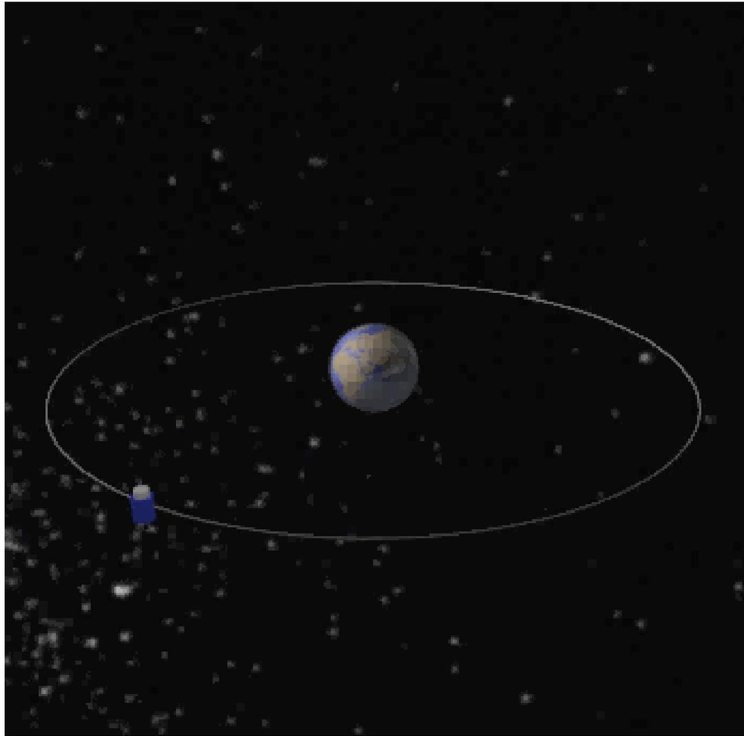
The geostationary orbit is quasi circular at 36000km altitude. One period lasts 24h, hence the satellite moves at the same angular speed as the Earth. The satellite seems fixed with respect to an observer on ground.
