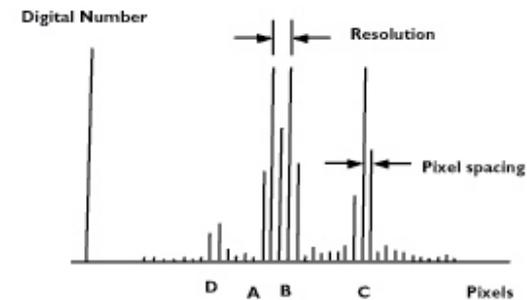
Resolution differs from pixel size, which is related to how densely the scene reflectivity has been sampled.
