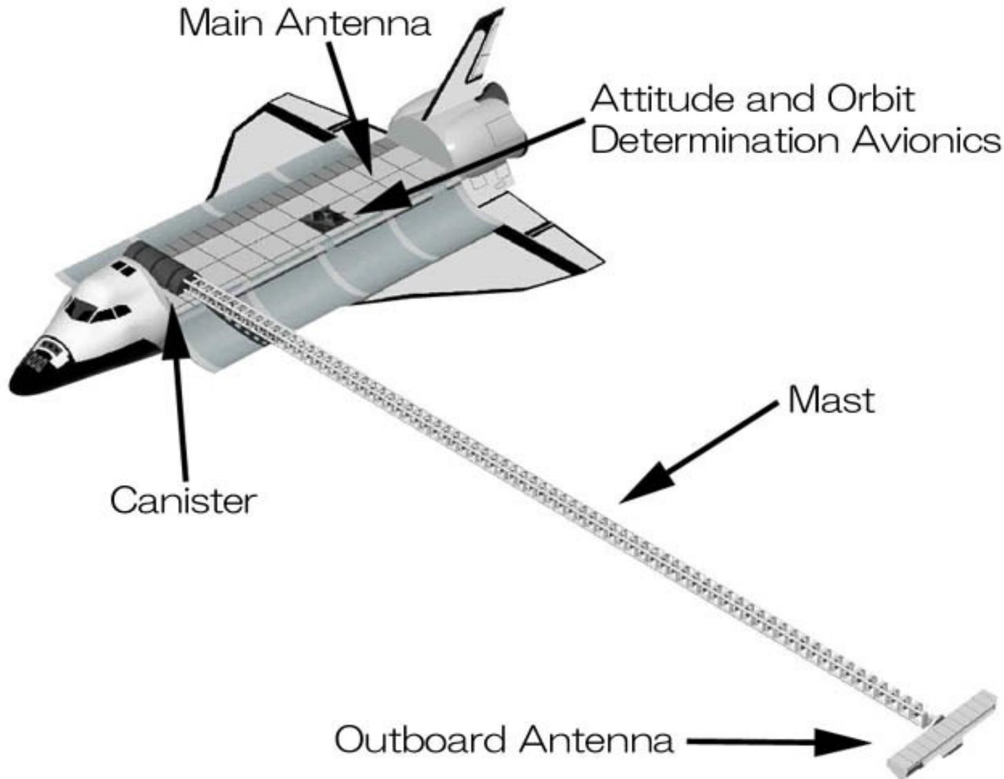
The Shuttle Radar Topography Mission (SRTM) obtained elevation data for a high-resolution digital topographic database of Earth. SRTM flew onboard the Space Shuttle Endeavour during an 11-day mission in February of 2000.
