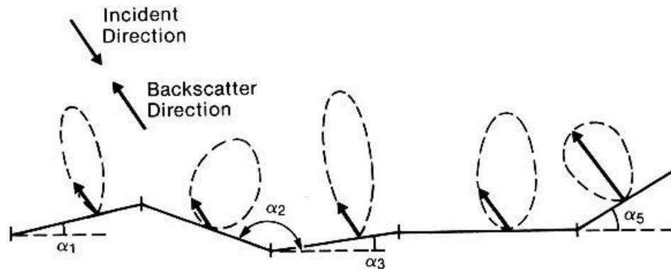
Scattering of a planar surface for slope angles
