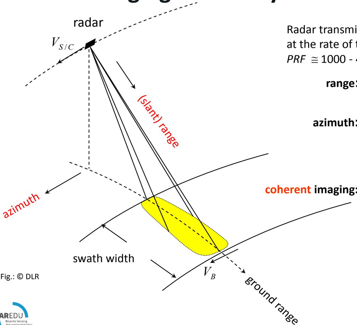
Radar transmits pulses and receives echoes at the rate of the pulse repetition frequency:  $PRF \cong 1000 - 4000 \text{ Hz}$
