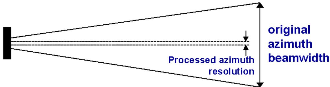
**This is the concept of Synthetic Aperture Radar – SAR**
