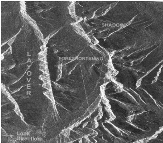
Layover is an extreme case of foreshortening, where the slope is bigger than the radar look angle ( $\theta$ ).
