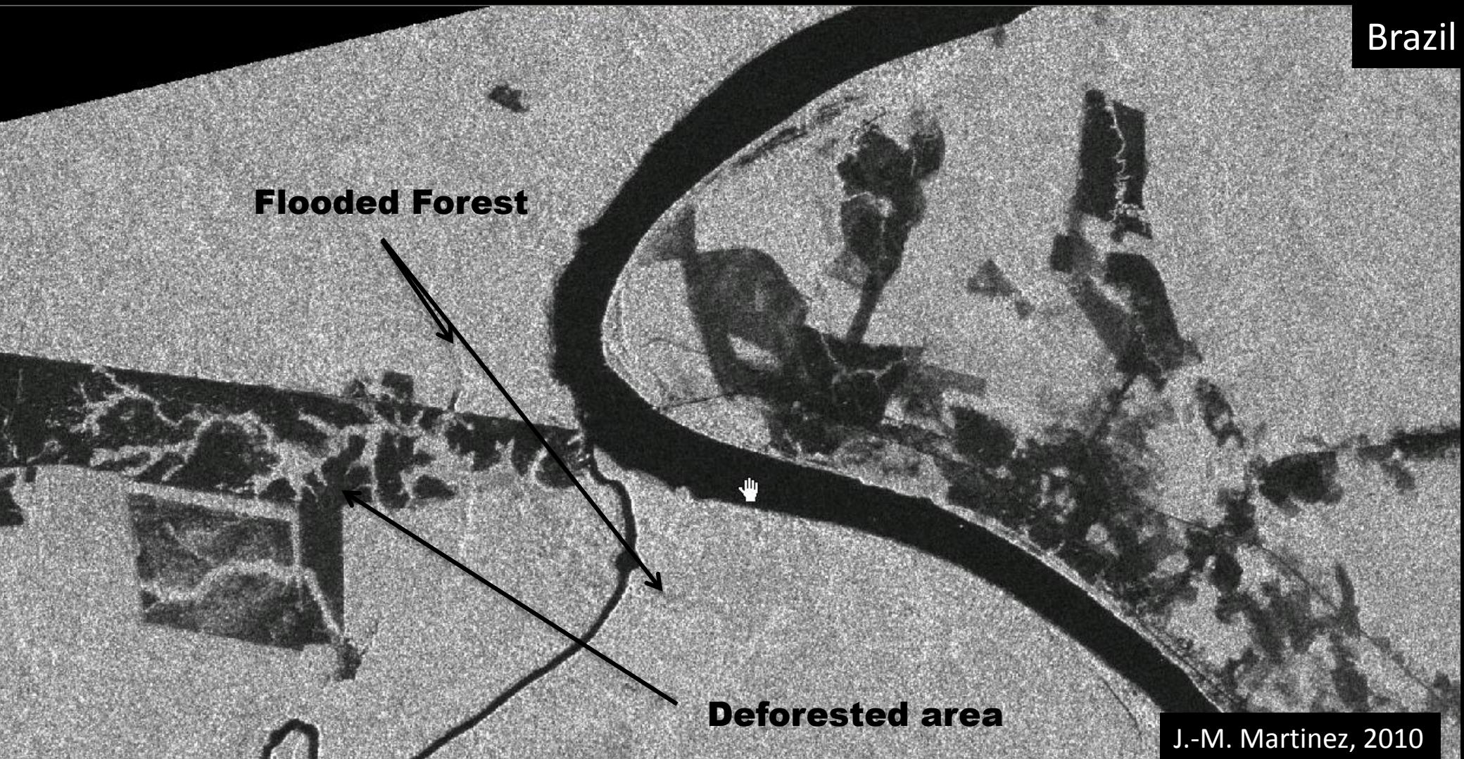
ALOS acquisition ( $\lambda = 24 \text{ cm}$ )- **HV** Polarization
