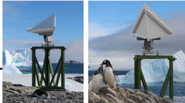
2 corner reflectors with known reference coordinates (< 5 mm)
