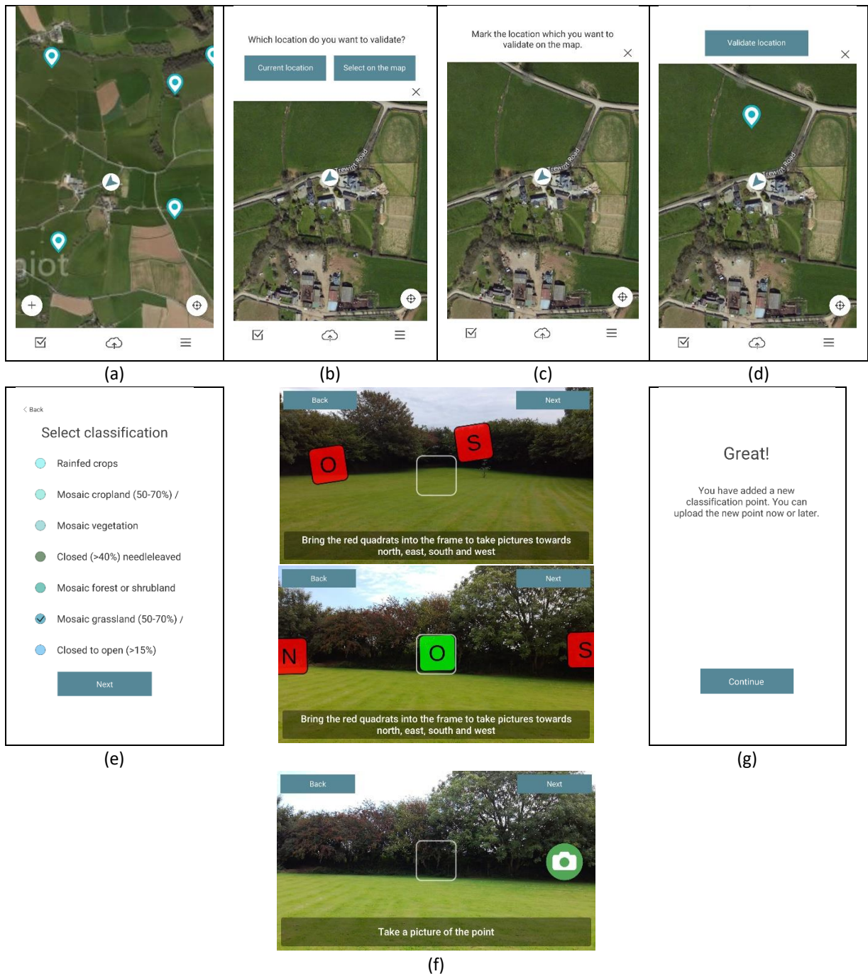
Figure 8: Opportunistic, in situ land cover data collection using LACO-Wiki Mobile. (a) Screen showing sample points (blue markers) and the + button on the bottom left; (b) After pressing +, the user is asked if they want to validate at their location or at a location to be selected on the map; (c) If select on the map is chosen, the user is asked to place a marker on the map; (d) Once the marker is placed, the user can add a land cover observation by pressing Validate location; (e) the user chooses the land cover type; (f) and then takes pictures in 4 cardinal directions; (g) a final screen is displayed informing the user that the point has been added.
