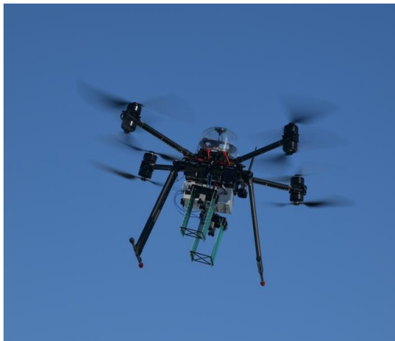
Drone equipped with an UWB Snow radar
