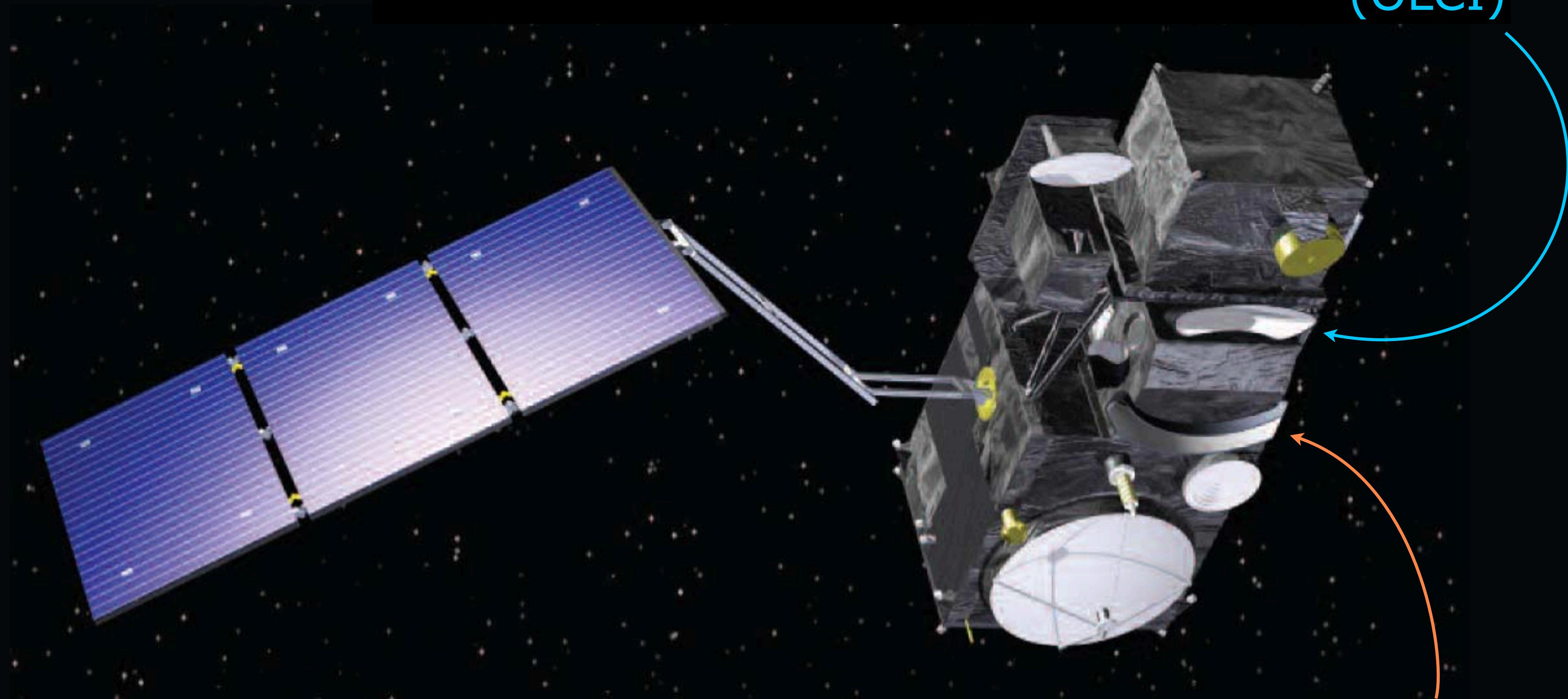
Sea and Land Surface Temperature Radiometer (SLSTR)
