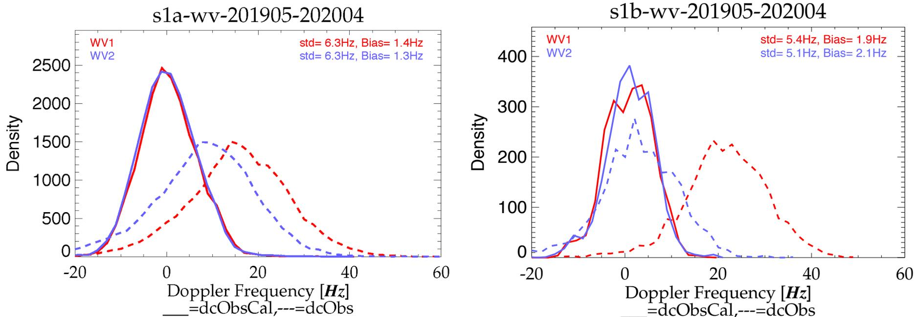
Figure: Histograms of S-1a (left) and S-1b (right) WV OCN RVL DC frequency before (---) and after (\_\_\_) calibration. The data was acquired between 1<sup>st</sup> May 2019 and 30<sup>th</sup> April 2020 over global land areas.
