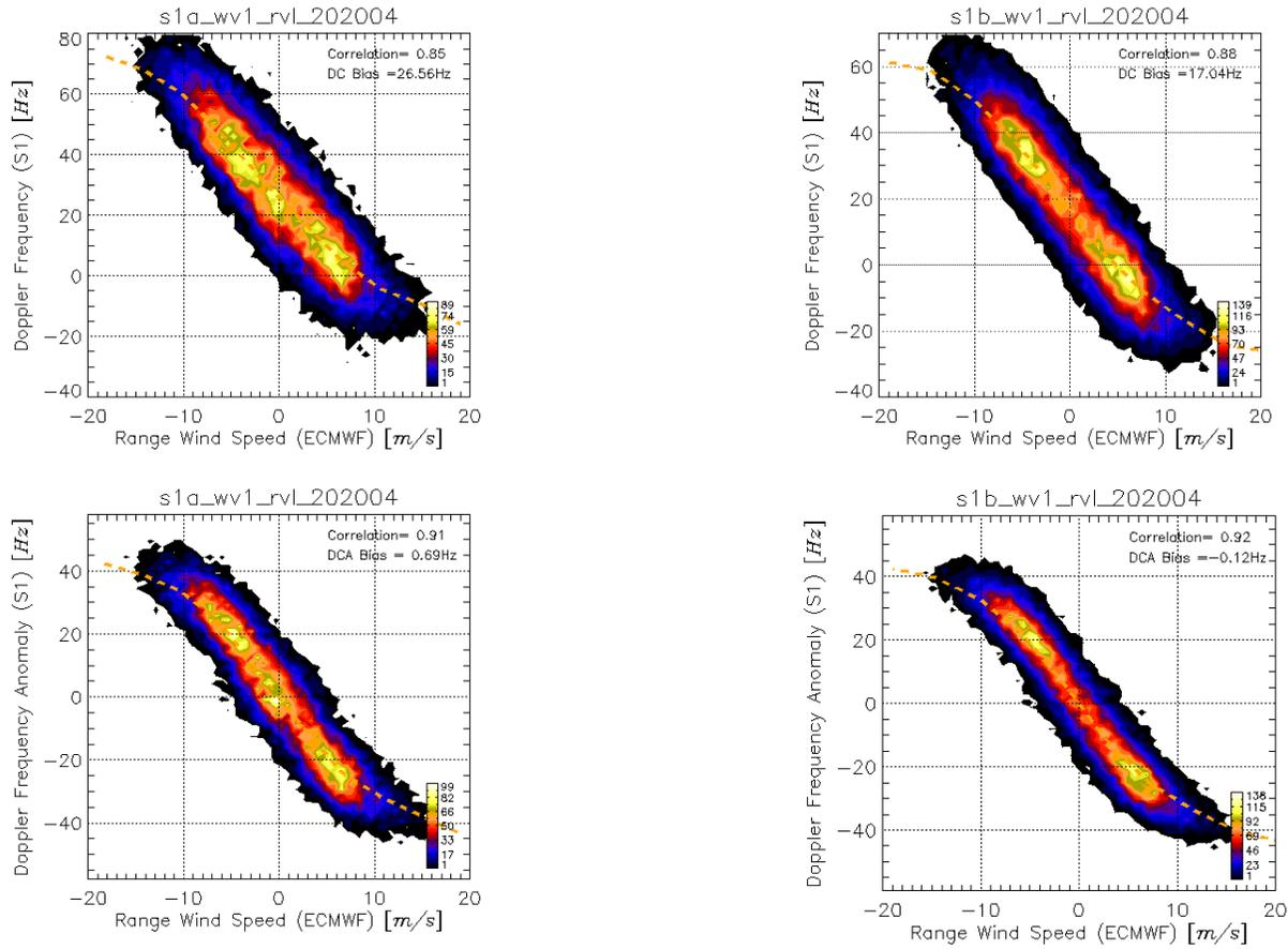
Figure : S-1a (left) and S-1b (right) WV Doppler frequency before (upper) and after (lower) calibration versus range wind speed (ECMWF).
