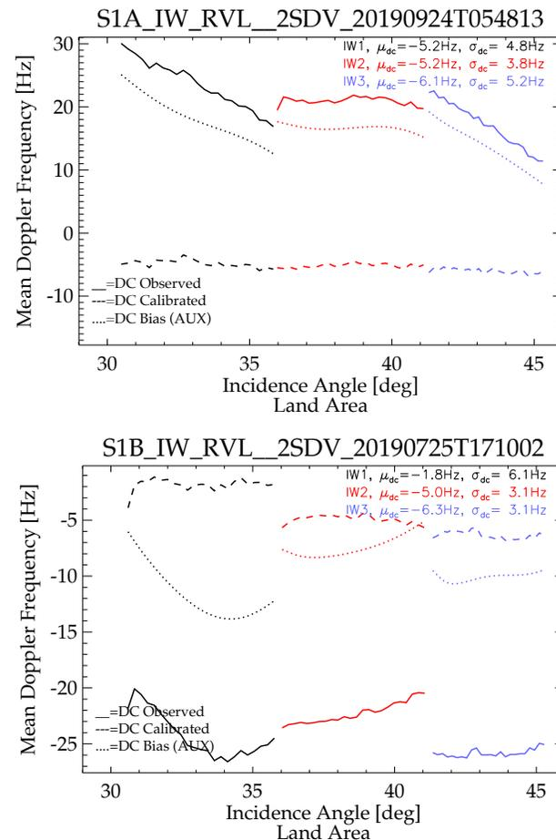
Figure: Mean DC profiles over swath (dcObs, dcObsCal, dcBias).
