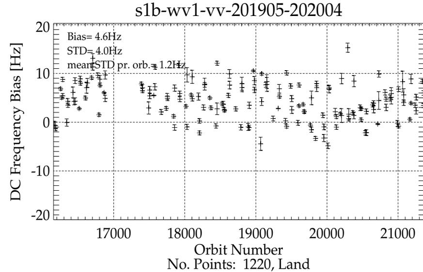
Figure : Examples of S-1a (a) and S-1b (b) WV mean calibrated DC pr. orbit segments over land areas. The vertical bars indicate the standard deviation over the orbit segment.
