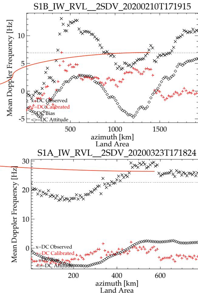
Figure: Mean DC profiles (dcObs, dcObsCal, dcAtt) along track.
