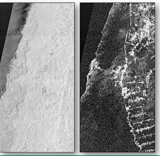
Fig.: ERS-Tandem intensity image and 1-day repeatpass phase coherence image (size 50 km by 100 km) (LUCKMAN et al., 2000).
