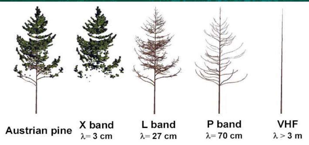
Fig. and Tab.: Main scatterers at different frequencies (Image credentials: THUY LE TOAN, Tab from LE TOAN ET AL., 2001).
