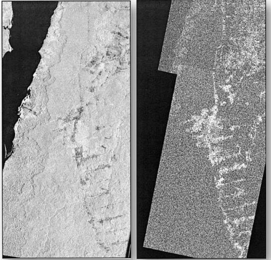
Fig.: JERS intensity image and 132-day repeat-pass phase coherence image (size 50 km by 100 km) (LUCKMAN et al., 2000).
