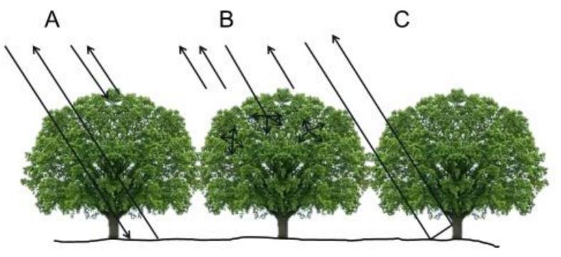
C - If the wave reflects off two surfaces before returning to the instrument, such as often arises in urban areas between ground and wall, or in forests between ground and tree trunks or between trunks and twigs, this is termed "double bounce".
