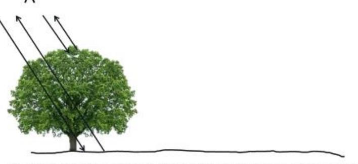
A - When a wave reflects off only one target and returns to the instrument this is known as direct scattering (or "single bounce"). This occurs when the wave hits a target that is at an orientation such that the wave is returned directly to the radar.
