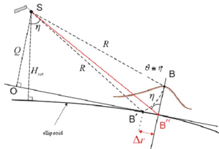
Point **B** with elevation **h** above the ellipsoid is imaged at position **B'** in SAR image, though its real position is **B''**. The offset  $\Delta r$  between **B'** and **B''** exhibits the effect of topographic distortions
