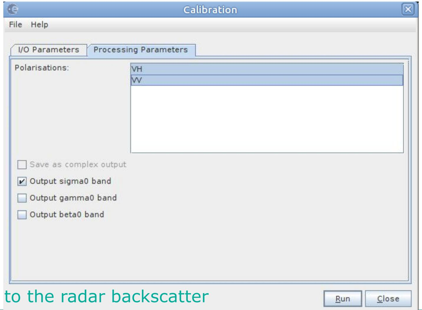
Pixel values can be directly related to the radar backscatter
