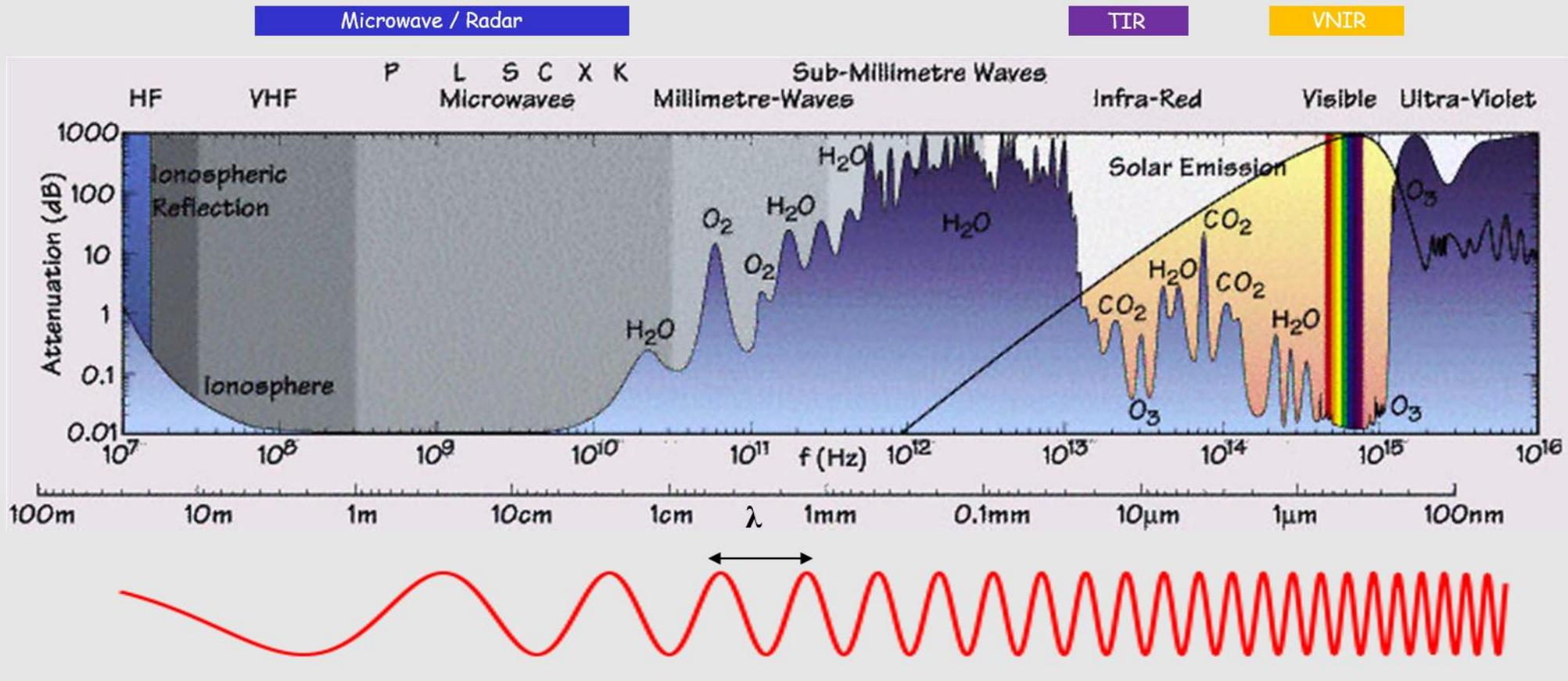
Electromagnetic spectrum and attenuation caused by Earth's atmosphere
