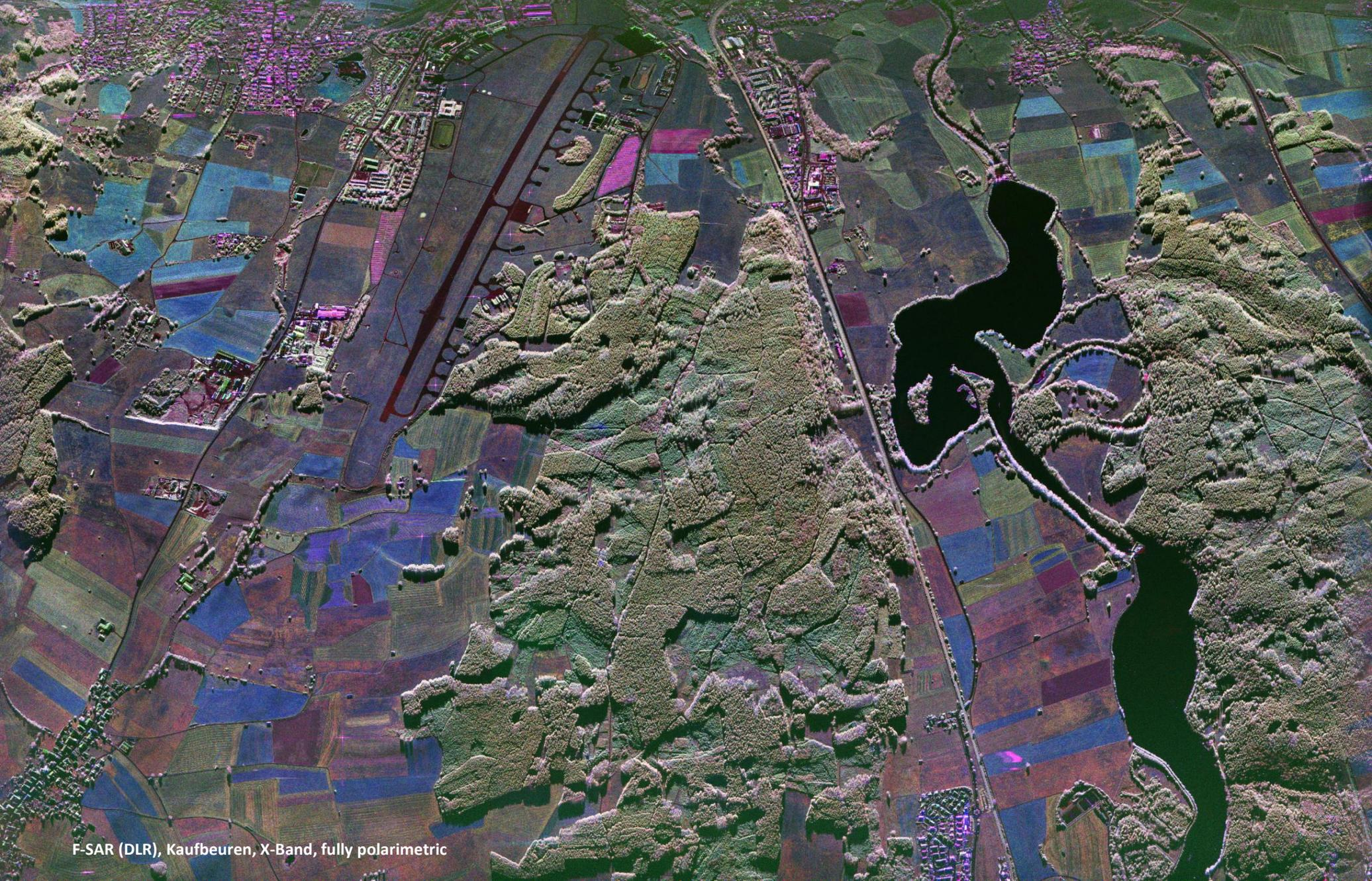
F-SAR (DLR), Kaufbeuren, X-Band, fully polarimetric
