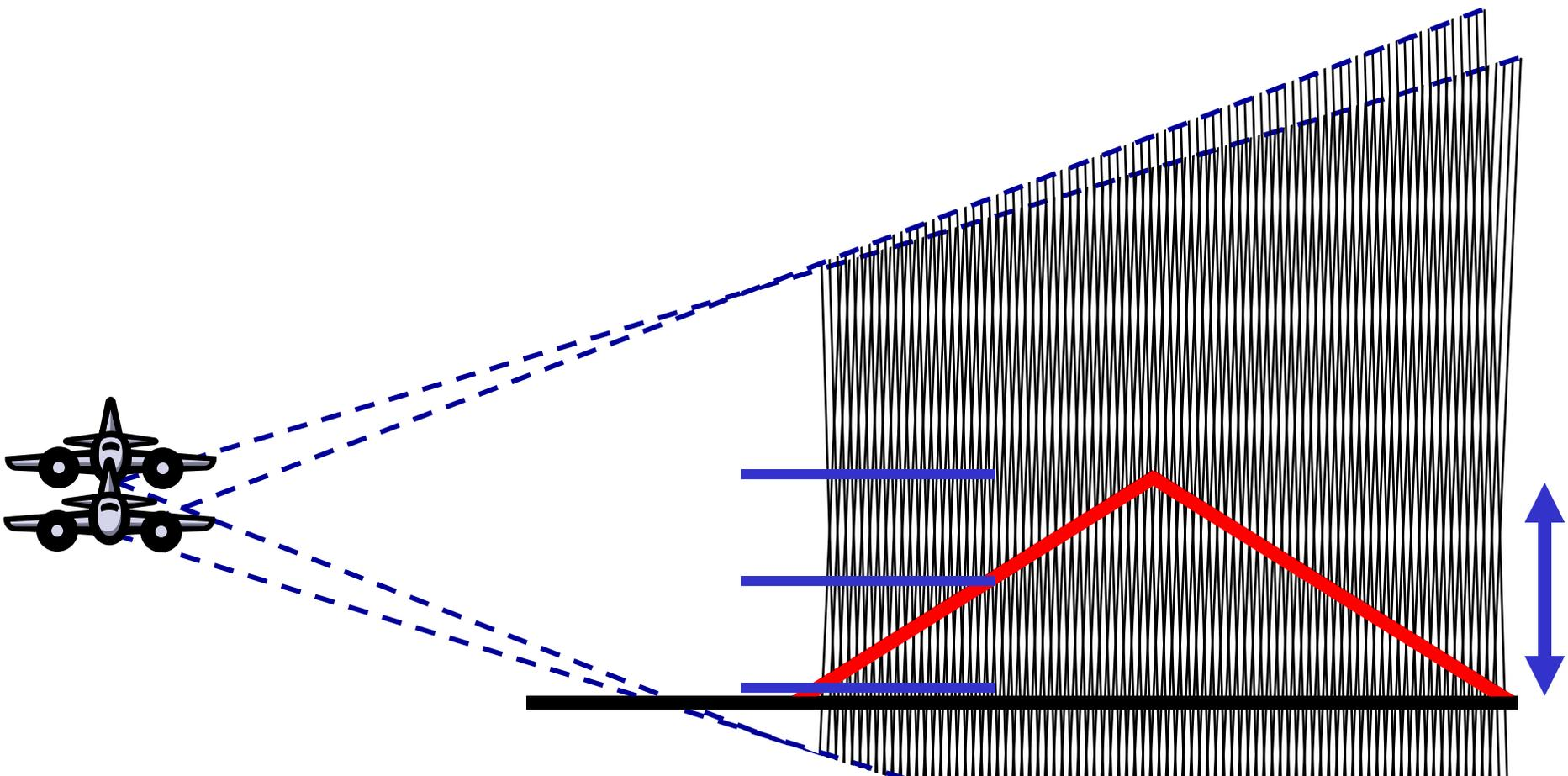
The Phase-to-Height Sensitivity increases with increasing the spatial baseline (i.e.  $\Delta\theta$  or  $B_{\perp}$ );
